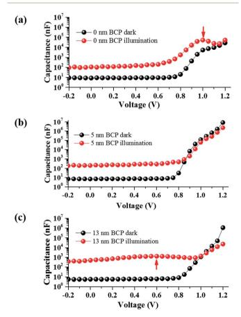
Fig. 5 C-V characteristics of the photovoltaic devices with 0 nm-BCP layer (a), 5 nm-BCP layer (b), 13 nm-BCP layer (c) under dark and illumination (LED white light, 60 mW cm<sup>-2</sup>). The frequency was set at 1 kHz.
