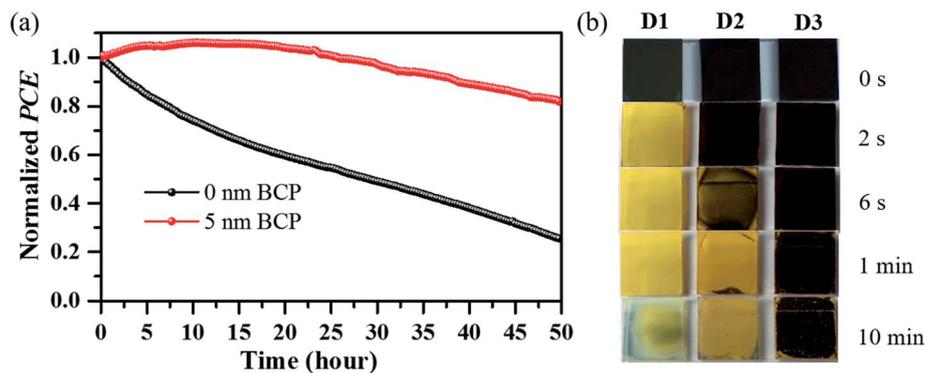
Fig. 6 (a) Normalized PCEs of the unencapsulated photovoltaic devices with 0 nm-BCP layer and 5 nm-BCP layer under continuous illumination (LED white light,  $60 \text{ mW cm}^{-2}$ ), kept in ambient air with controlled humidity of  $\sim 30\%$ . (b) Comparison of degradation speeds from three different samples: (D1) FTO/perovskite, (D2) FTO/perovskite/PCBM, (D3) FTO/perovskite/PCBM/BCP, the samples were all soaked in water for 10 minutes at room temperature.
