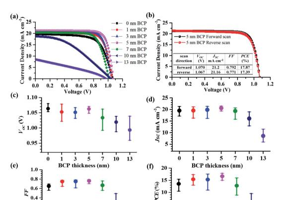
Fig. 2 (a) The forward scan J-V curves of PSCs with varying BCP layer thicknesses, measured under simulated solar light (AM 1.5G, 100 mW cm<sup>-2</sup>). (b) J-V curves of the champion device with a BCP layer thickness of 5 nm. Dependences of (c) open-circuit voltage ( $V_{OC}$ ), (d) short-circuit photocurrent density ( $J_{SC}$ ), (e) fill factor (FF), (f) PCE on the corresponding thickness of BCP layer, 10 samples being included.
