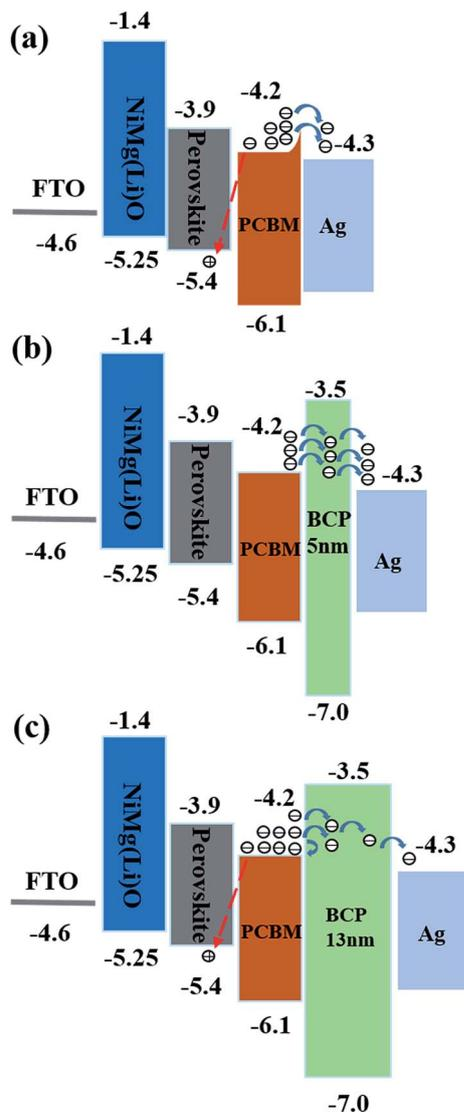
Fig. 4 The energy diagram and charge transport mechanism of photovoltaic devices with varied BCP thicknesses, (a) device with 0 nm-BCP layer, (b) device with 5 nm-BCP layer, (c) device with 13 nm-BCP layer.
