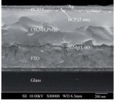
Fig. 1 (a) The device structure of FTO/NiMg(Li)O/CH<sub>3</sub>NH<sub>3</sub>PbI<sub>3</sub>/PCBM/BCP/Ag. (b) A high-resolution cross-sectional scanning electron microscopy (SEM) image of photovoltaic device with 5 nm-BCP buffer layer.
