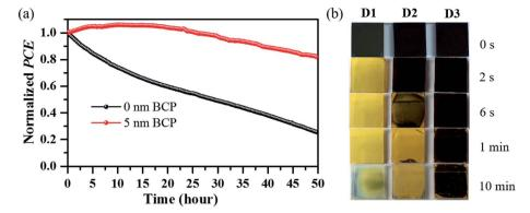
Fig. 6 (a) Normalized PCEs of the unencapsulated photovoltaic devices with 0 nm-BCP layer and 5 nm-BCP layer under continuous illumination (LED white light, 60 mW cm $^{-2}$ ), kept in ambient air with controlled humidity of  $\sim 30\%$ . (b) Comparison of degradation speeds from three different samples: (D1) FTO/perovskite, (D2) FTO/perovskite/PCBM, (D3) FTO/perovskite/PCBM/BCP, the samples were all soaked in water for 10 minutes at room temperature.
