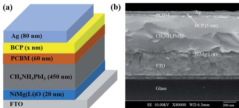
Fig. 1 (a) The device structure of FTO/NiMg(Li)O/CH<sub>3</sub>NH<sub>3</sub>PbI<sub>3</sub>/PCBM/BCP/Ag. (b) A high-resolution cross-sectional scanning electron microscopy (SEM) image of photovoltaic device with 5 nm-BCP buffer layer.
