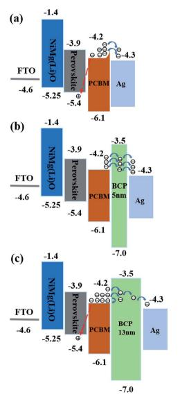
Fig. 4 The energy diagram and charge transport mechanism of photovoltaic devices with varied BCP thicknesses, (a) device with 0 nm-BCP layer, (b) device with 5 nm-BCP layer, (c) device with 13 nm-BCP layer.
