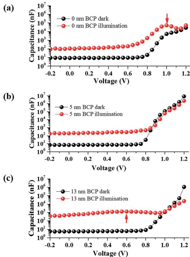
Fig. 5  $C-V$  characteristics of the photovoltaic devices with 0 nm-BCP layer (a), 5 nm-BCP layer (b), 13 nm-BCP layer (c) under dark and illumination (LED white light,  $60 \text{ mW cm}^{-2}$ ). The frequency was set at 1 kHz.
