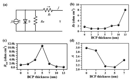
Fig. 3 (a) The single-diode equivalent circuit model of the studied PSC, the dependences of the fitted parameters including (b) R<sub>S</sub>, (c) R<sub>SH</sub>, (d) A on the BCP layer thickness.
