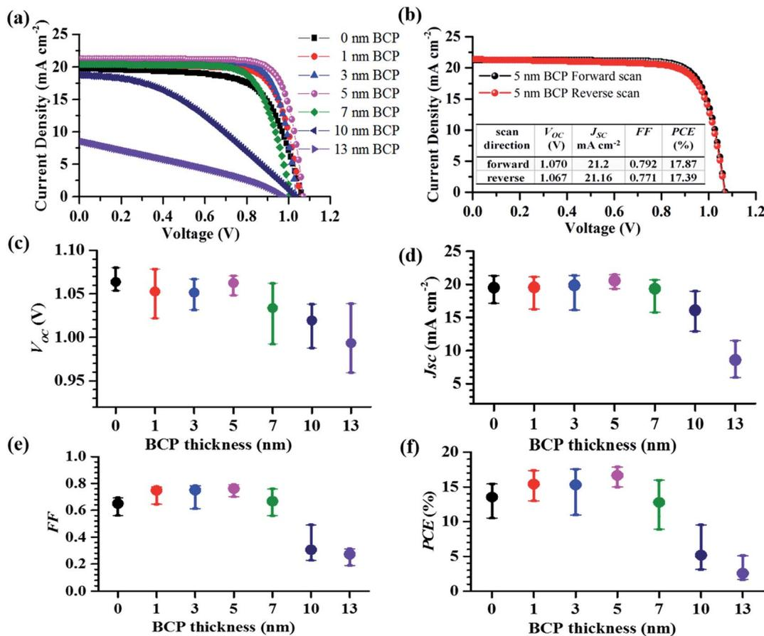
Fig. 2 (a) The forward scan  $J$ - $V$  curves of PSCs with varying BCP layer thicknesses, measured under simulated solar light (AM 1.5G, 100 mW cm<sup>-2</sup>). (b)  $J$ - $V$  curves of the champion device with a BCP layer thickness of 5 nm. Dependences of (c) open-circuit voltage ( $V_{OC}$ ), (d) short-circuit photocurrent density ( $J_{SC}$ ), (e) fill factor (FF), (f) PCE on the corresponding thickness of BCP layer, 10 samples being included.
