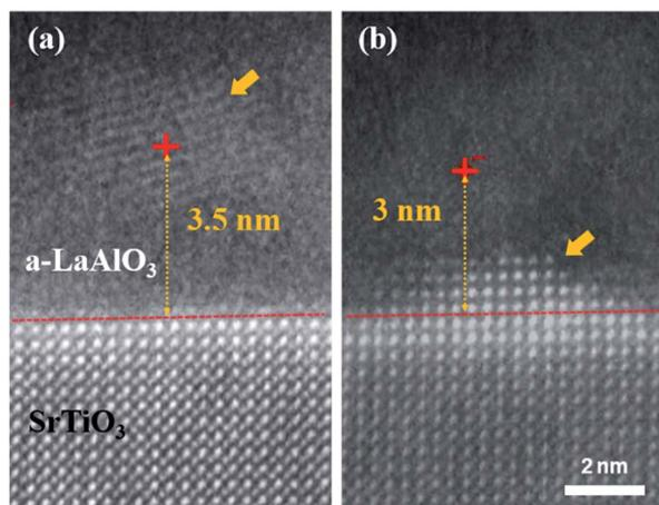
Fig. 2 HAADF STEM images of a-LAO/STO irradiated with a convergent e-beam (a) 3.5 nm and (b) 3 nm away from the interface. The specimen was irradiated at an electron dose rate of  $0.169 \times 10^9 \text{ e}^- \text{ \AA}^{-1} \text{ s}^{-1}$  for 60 s, and the current of the e-beam was 0.34 nA. The dashed red lines are guidelines, which are the starting points for crystallization, and the yellow arrows indicate the crystallized LAO region.
