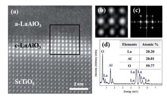
Fig. 1 (a) HAADF STEM image showing that an LAO crystal has grown from the STO substrate under e-beam irradiation. (b) Filtered atomic-column image of a crystallized LAO region. An Al atomic column with a low intensity due to its low atomic weight is visible. (c) FFT pattern acquired from the black square marked in (a). (d) EDS spectrum with the quantitative chemical composition (inset table), which was obtained from the LAO crystal.
