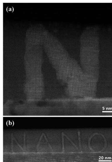
Fig. 6 HAADF STEM images of patterned letters onto a-LAO region using e-beam irradiation. The pattern keeps the coherent atomic structure from the STO<sub>3</sub> crystalline substrate.
