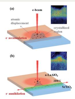
Fig. 5 Schematics showing the distribution of electrons around the incident e-beam in the a-LAO overlayer. (a) The incident electrons accumulate when the interface is insulating. (b) The negative charges are dissipated through the conductive interface, which acts as a bottom electrode. The inset images are colored HRSTEM images of Fig. 3a and b showing the crystallization kinetics and shape.
