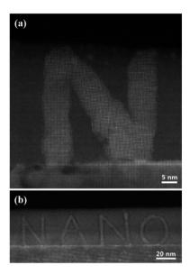
Fig. 6 HAADF STEM images of patterned letters onto a-LAO region using e-beam irradiation. The pattern keeps the coherent atomic structure from the  $STO_3$  crystalline substrate.
