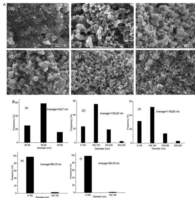
Fig. 4 SEM micrographs (A) and size (B) of nanocomposites prepared at 75 °C under different pH: (a)  $\text{SiO}_2$ , (b) lignin, (c) LS1, (d) LS2, (e) LS3 and (f) LS4.
