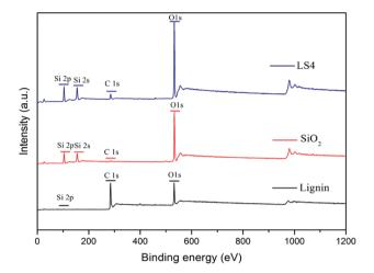
Fig. 1 XPS patterns of lignin, LS4 and silical
