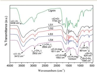
Fig. 2 FT-IR spectra of lignin and lignin/silica nanocomposites.
