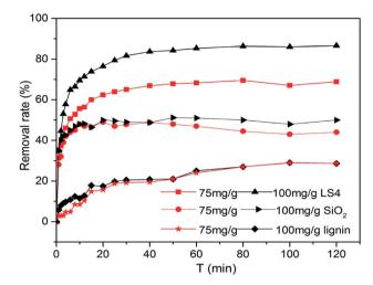
Fig. 6 Removal rate of methylene blue at different concentrations (75 and 100 mg  $g^{-1}$ ) of LS4, silica and lignin.
