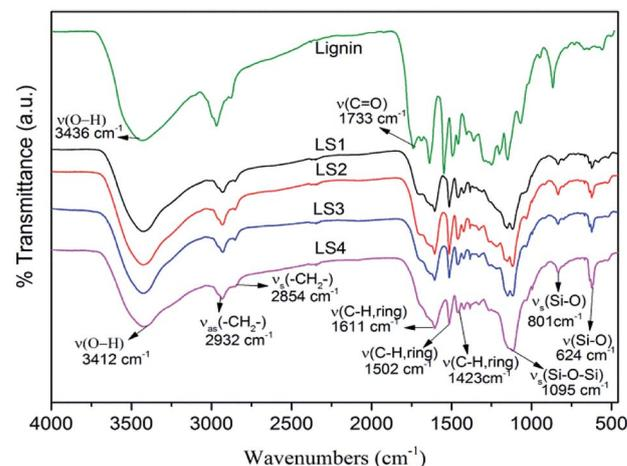
Fig. 2 FT-IR spectra of lignin and lignin/silica nanocomposites.
