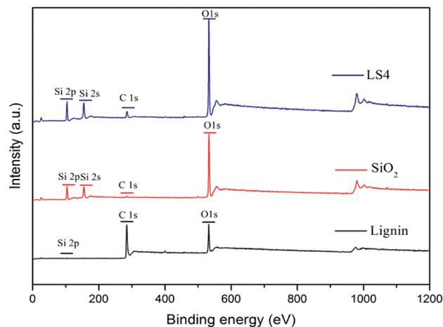
Fig. 1 XPS patterns of lignin, LS4 and silica.
