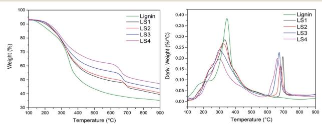
Fig. 3 TGA and DTGA of lignin and composites prepared at different pH.
