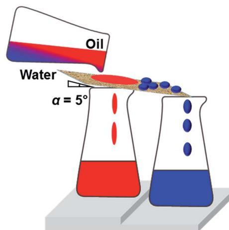
Fig. 9 Schematic illustration of oil–water separation by a metal mesh coated with modified CNF. The mesh pore size was 150  $\mu$ m. The water droplet easily bounces and rolls off at a sliding angle 5° while oil penetrates through the mesh by gravitational force.
