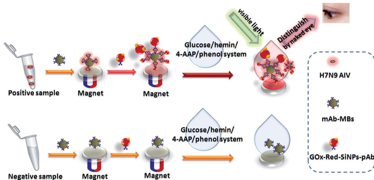
Fig. 2 Schematic view of optical MB-MEMSCI for rapid detection of H7N9.
