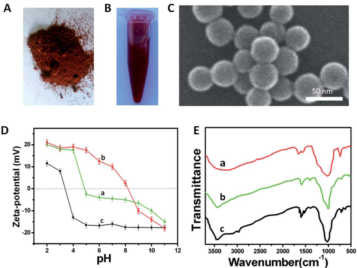
Fig. 3 Digital photos of Red-SiNPs (A) and their aqueous solution (B). SEM image of Red-SiNPs (C). Zeta potential (D) of Red-SiNPs (a), Red-SiNPs-NH<sub>3</sub> (b), Red-SiNPs-COOH (c). FTIR spectra (E) of Red-SiNPs (c), Red-SiNPs-NH<sub>3</sub> (b), and Red-SiNPs-COOH (a).
