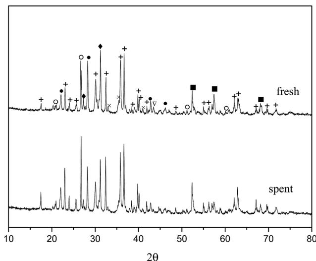
Fig. 15 XRD patterns of fresh and spent TF-Ni/olivine catalysts +: Mg<sub>2</sub>SiO<sub>4</sub>; ◆: MgSiO<sub>3</sub>; ○: (Fe,Ni); ×: Fe<sub>2</sub>O<sub>3</sub>; ●: (Mg,Fe)SiO<sub>3</sub>; ▽: Ni; ■: (Ni,Mg)<sub>2</sub>SiO<sub>4</sub>.
