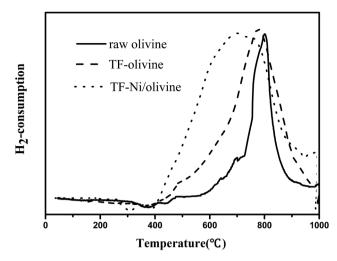
Fig. 6 H<sub>2</sub>-TPR of differently treated olivine catalysts.
