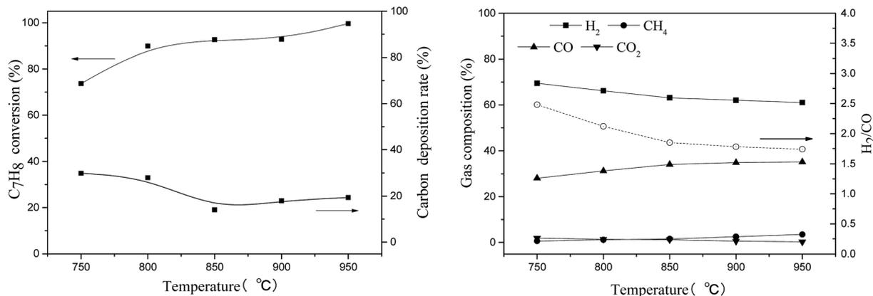
Fig. 9 Effect of reaction temperature on toluene steam reforming using TF-Ni/olivine (S/C = 0.73, WHSV = 0.9 h<sup>-1</sup>).
