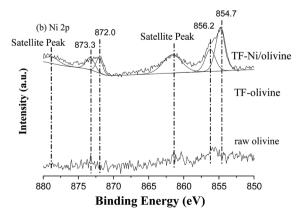
Fig. 5 X-ray photoelectron spectra of differently treated olivine catalysts: effects of (a) Fe 2p and (b) Ni 2p.
