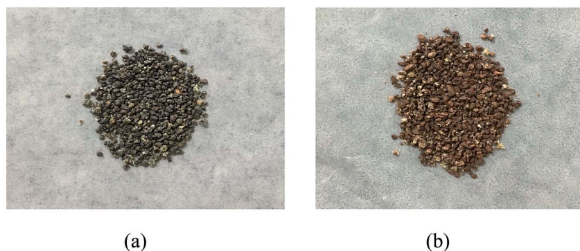
Fig. 12 Intuitive morphology of the TF-Ni/olivine catalysts: (a) fresh TF-Ni/olivine (b) spent TF-Ni/olivine.
