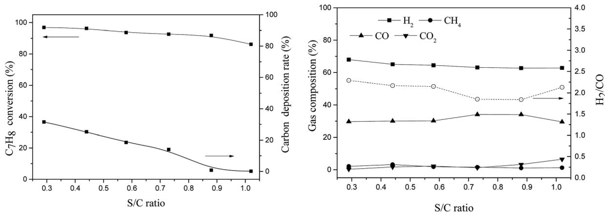
Fig. 11 Effect of the S/C ratio on toluene steam reforming using TF-Ni/olivine (reaction temperature of 850 °C, WHSV = 0.9 h<sup>-1</sup>).
