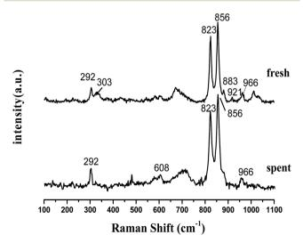
Fig. 16 Laser Raman spectra of fresh and spent TF-Ni/olivine catalysts.
