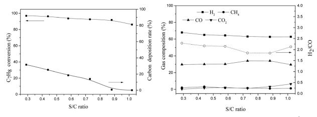
Fig. 11 Effect of the S/C ratio on toluene steam reforming using TF-Ni/olivine (reaction temperature of 850 °C, WHSV =  $0.9 h^{-1}$ ).
