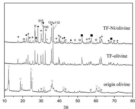
Fig. 3 XRD patterns of differently treated olivine catalysts. +:  $\text{Mg}_2\text{SiO}_4$ ; ◆:  $\text{MgSiO}_3$ ; ○: (Fe,Ni); ×:  $\text{Fe}_2\text{O}_3$ ; ∇: Ni; □:  $\text{Mg}_3\text{Si}_2\text{O}_5(\text{OH})_4$ ; ⊗:  $\text{MgFe}_2\text{O}_4$ ; ■:  $(\text{Ni,Mg})_2\text{SiO}_4$ .
