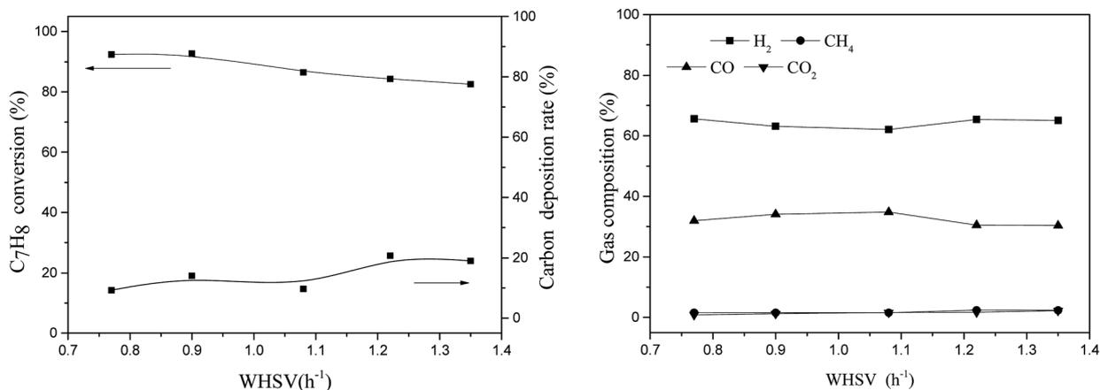
Fig. 10 Effect of WHSV on toluene steam reforming using TF-Ni/olivine (reaction temperature of 850 °C, S/C = 0.73).
