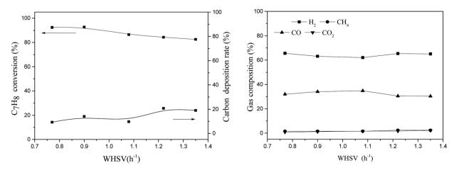
Fig. 10 Effect of WHSV on toluene steam reforming using TF-Ni/olivine (reaction temperature of 850  $^{\circ}$ C, S/C = 0.73).
