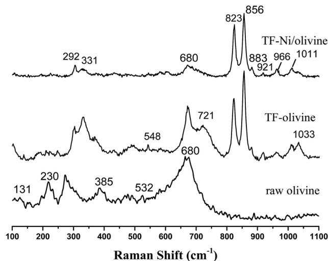
Fig. 4 Laser Raman spectra of differently treated olivine catalysts.
