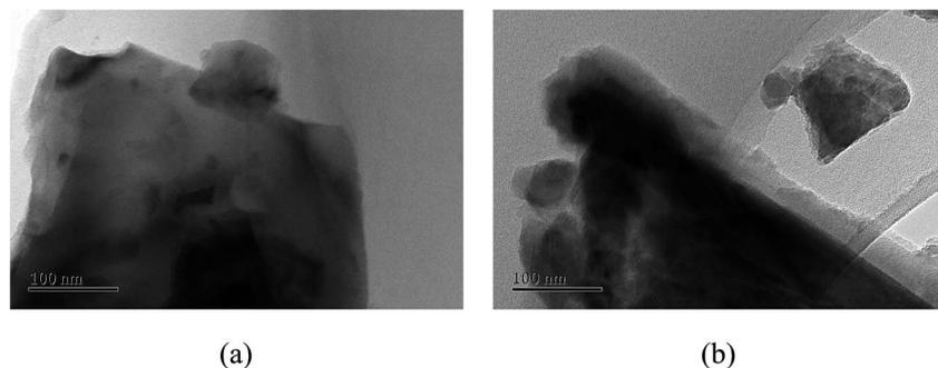
Fig. 14 TEM images of fresh and spent TF-Ni/olivine catalysts: (a) fresh TF-Ni/olivine (b) spent TF-Ni/olivine.
