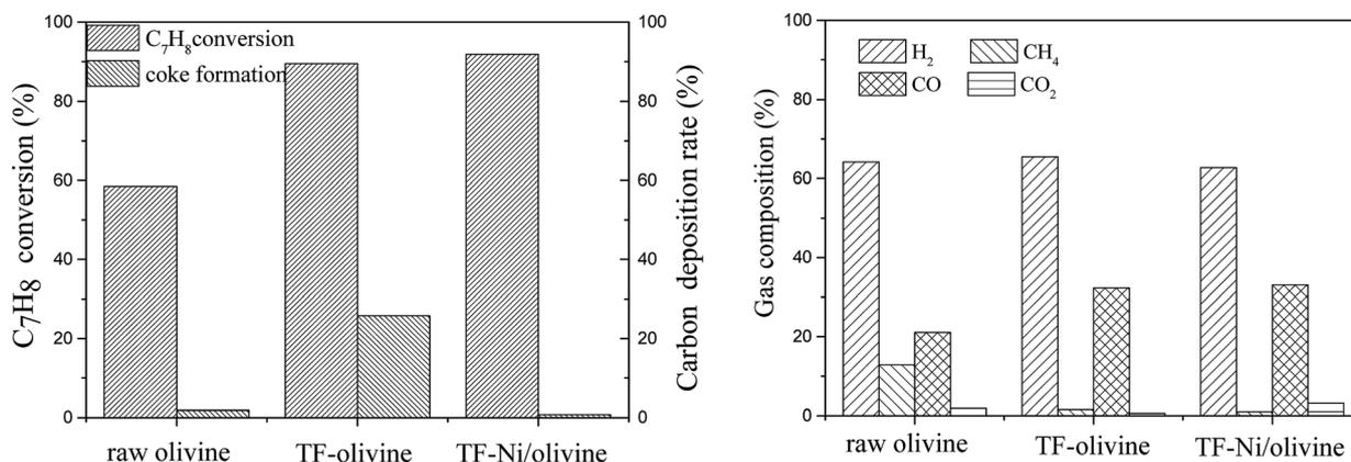
Fig. 8 Effects of three olivine catalysts on toluene/H<sub>2</sub>O reforming (reaction temperature of  $850^\circ\text{C}$ , S/C = 0.88, WHSV =  $0.9\text{ h}^{-1}$ ).
