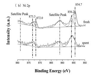
Fig. 17 X-ray photoelectron spectra of fresh and spent TF-Ni/olivine catalysts: (a) Fe 2p, (b) Ni 2p.
