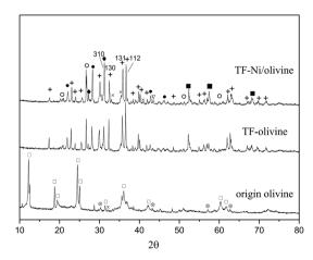
Fig. 3 XRD patterns of differently treated olivine catalysts. +: Mg<sub>2</sub>SiO<sub>4</sub>;
