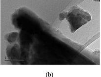
Fig. 14 TEM images of fresh and spent TF-Ni/olivine catalysts: (a) fresh TF-Ni/olivine (b) spent TF-Ni/olivine.
