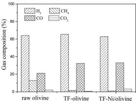
Effects of three olivine catalysts on toluene/ $H_2O$  reforming (reaction temperature of 850 °C, S/C = 0.88, WHSV = 0.9 h<sup>-1</sup>).
