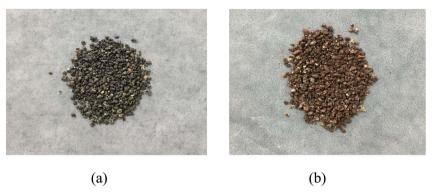
Fig. 12 Intuitive morphology of the TF-Ni/olivine catalysts: (a) fresh TF-Ni/olivine (b) spent TF-Ni/olivine.
