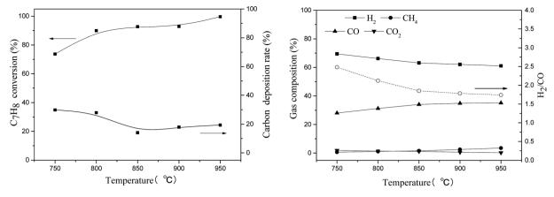
Effect of reaction temperature on toluene steam reforming using TF-Ni/olivine (S/C = 0.73, WHSV =  $0.9 h^{-1}$ )
