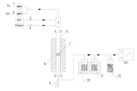
Fig. 1 Experimental scheme of  $C_7H_8/H_2O$  reforming. (1, 2) Mass flowmeter, (3, 4) peristaltic pump, (5) commingler (6) quartz reactor, (7) catalyst, (8) furnace, (9) thermocouple, (10) condenser, (11) isopropanol, (12) dryer.
