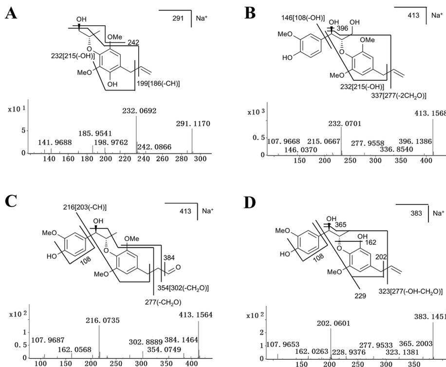
Fig. 6 Tandem MS spectra and fragmentation pattern of some representative metabolites of MRL. (A) Tandem MS spectra and chemical structure of **M2**. (B) Tandem MS spectra and chemical structure of **M6**. (C) Tandem MS spectra and chemical structure of **M8**. (D) Tandem MS and chemical structure of **M11**. MS/MS fragmentation was conducted with collision energy at 20 eV.
