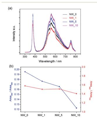
Fig. 5 (a) Photoluminescence (PL) spectra of ZnO NWs and (b) the change of ratio of peak area at 380 nm to area at 560 nm ( $R_1$ ), and peak area at 380 nm to area at 750 nm ( $R_2$ ).
