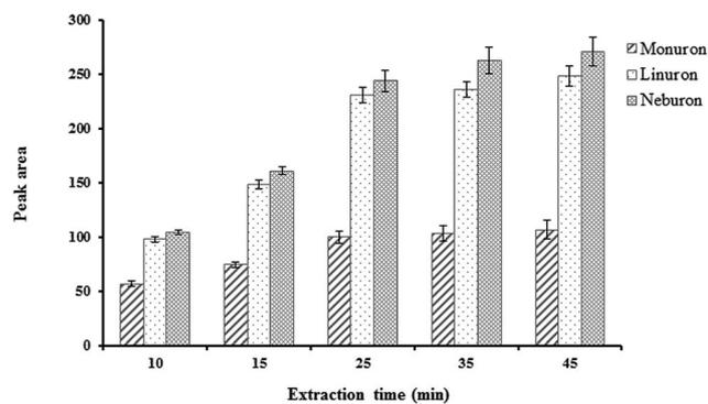
Fig. 4 Effect of extraction time on the extraction efficiency of phenylurea herbicides (analyte concentration:  $5 \mu\text{g L}^{-1}$ ; sample volume: 15.0 mL; desorption time: 5 min; shaking rate for extraction: 210 rpm; shaking rate for desorption: 210 rpm; volume of desorption solvent: 200  $\mu\text{L}$  and desorption solvent: 2-propanol).
