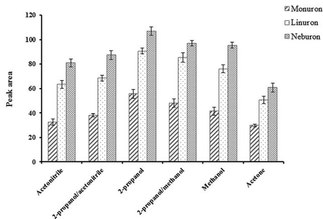
Fig. 3 Effect of solvent type on the extraction efficiency of phenylurea herbicides (analyte concentration:  $5 \mu\text{g L}^{-1}$ ; sample volume: 15.0 mL; shaking rate for extraction: 210 rpm; shaking rate for desorption: 210 rpm; extraction time: 15 min; desorption time: 10 min and volume of desorption solvent: 150  $\mu\text{L}$ ).
