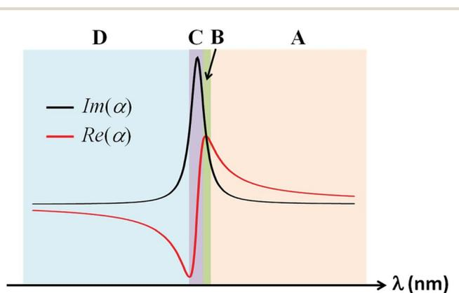
Fig. 6 Spectral dependence of the dispersively shaped real part of the complex polarizability ( $\text{Re}(\alpha)$ ) and the Lorentzian-shaped imaginary counterpart ( $\text{Im}(\alpha)$ ) shown in red and black curves. The regions highlighted with different colors represent spectral regions with distinct relative magnitudes between the real and the imaginary part of the complex polarizability.
