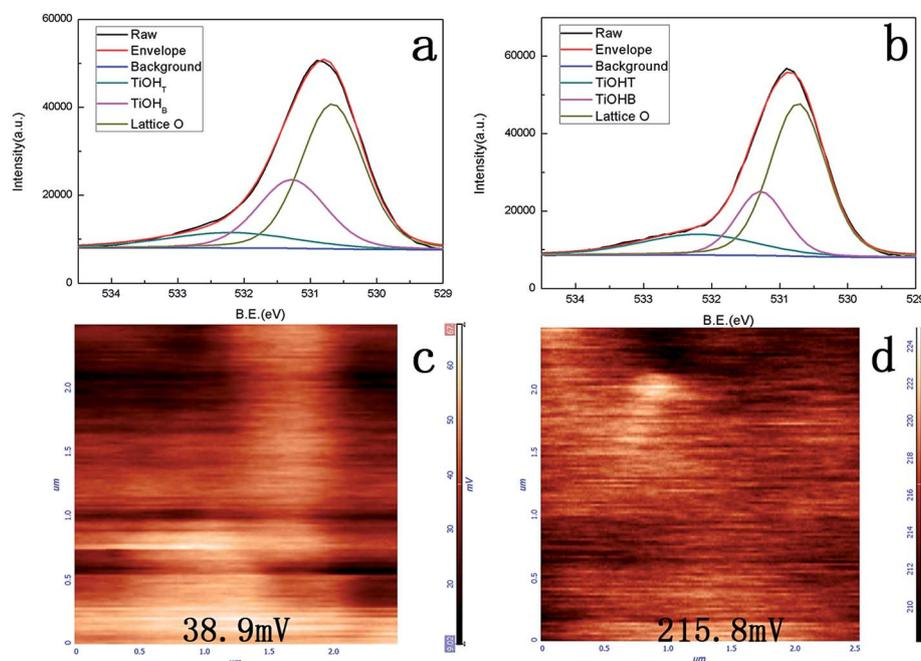
Fig. 3 XPS spectra of the TiO<sub>2</sub> nanowire films: (a) O 1s of the H<sub>2</sub>Ti<sub>3</sub>O<sub>7</sub> nanowire film, (b) O 1s of the anatase nanowire film; KFM of the (c) H<sub>2</sub>Ti<sub>3</sub>O<sub>7</sub> nanowire film and (d) anatase nanowire film.
