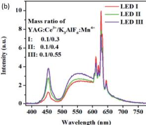
Fig. 8 (a) Concentration dependent emission spectra of  $K_3AlF_6$ :Mn<sup>4+</sup>. (b) Electroluminescence spectra of prototype LEDs, employing  $K_3AlF_6$ :Mn<sup>4+</sup> as the red converter component, commercial yellow YAG:Ce<sup>3+</sup> and a blue InGaN chip at a 40 mA drive current.<sup>42</sup>
