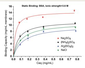
Fig. 6 The effects of salt type on the binding of BSA to PCVL grafted membrane substrates in 3.6 M ion strength Na<sub>2</sub>SO<sub>4</sub>, (NH<sub>4</sub>)<sub>2</sub>SO<sub>4</sub>, Al<sub>2</sub>(SO<sub>4</sub>)<sub>3</sub> and NaCl solutions. The isotherm fitting is based on Langmuir model.
