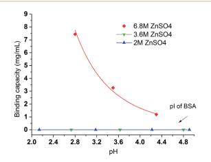
Fig. 7 The pH effects of BSA binding under various ionic strength of ZnSO $_4$ . All results were averaged by two replicates conducted under the same binding condition. Initial BSA concentration was kept at 0.09 mg mL $^{-1}$ . The fitted line just serves as a visual guide.
