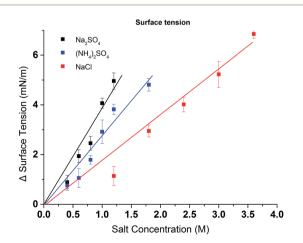
Fig. 4 Excess surface tension of (NH<sub>4</sub>)<sub>2</sub>SO<sub>4</sub>, Na<sub>2</sub>SO<sub>4</sub> and NaCl at various concentrations (water surface tension is 73.54  $\pm$  0.16 mN m<sup>-1</sup>). All data were averaged by five measurements.
