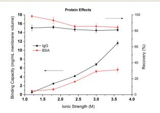
Fig. 9 Dynamic binding capacities and recoveries of IgG<sub>4</sub> and BSA as a function of the ionic strength of Na<sub>2</sub>SO<sub>4</sub>
