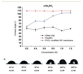
Fig. 5 Salt concentration effects on contact angle of HIC membranes at  $\rm Na_2SO_4$  concentration ranging from 0.2 M to 1.2 M. The average results of five random locations were reported here (a and b) with two other non-responsive surfaces as controls.
