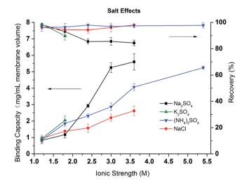
Fig. 10 The effects of salt and ionic strength on the dynamic binding capacity and recovery of BSA on PVCL modified membrane substrate.
