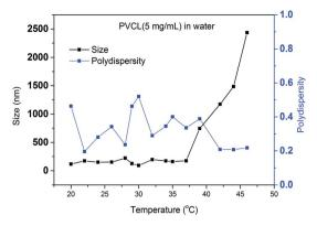
Fig. 2 Size measurement of synthesized PVCL under different temperatures bv dynamic light scattering and calculated polydispersity.
