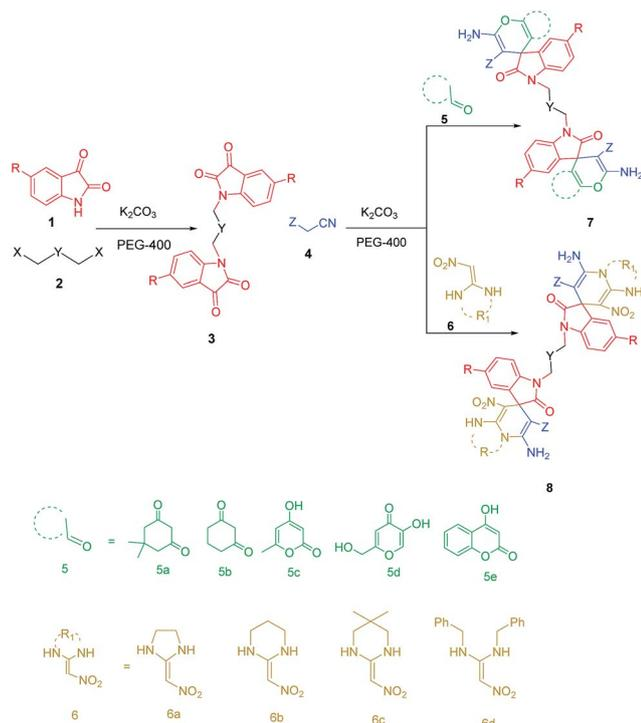
Scheme 1 The one-pot, multi-component synthesis of bis-spirooxindoles in PEG-400/ $K_2CO_3$  at room temperature.
