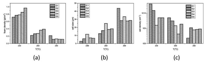
Fig. 3 Effect of gel content on (a) foam density, (b) average cell size, and (c) cell density of PEK-C foams (saturation time: 2 h; pressure: 12 MPa).
