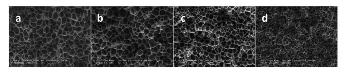
Fig. 8 SEM images of PEK-C foams (S3) prepared at 280  $^{\circ}$ C and different pressure levels: (a) 8 MPa; (b) 10 MPa; (c) 12 MPa and (d) 16 MPa (scale bar 100  $\mu$ m).
