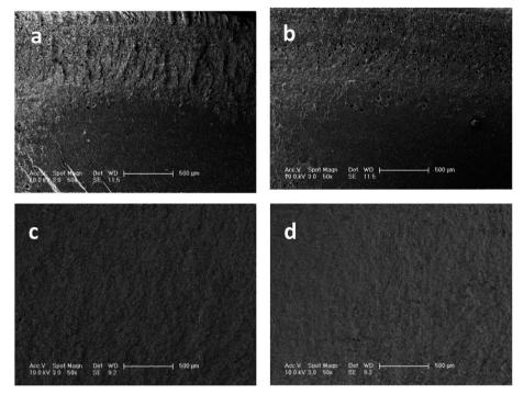
Fig. 4 SEM images of PEK-C foams prepared at 230 °C after different absorption times: (a) 0.5 h, (b) 1 h, (c) 2 h, and (d) 3 h.
