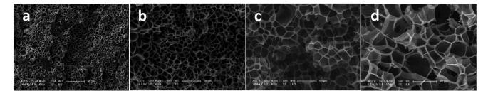
Fig. 6 SEM images of PEK-C foams (S2) prepared at 12 MPa and at different temperatures: (a) 230 °C; (b) 250 °C; (c) 280 °C; and (d) 300 °C (scale bar: 50  $\mu$ m).
