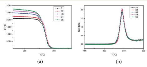
Fig. 1 Storage modulus (a) and  $\tan \delta$  (b) of PEK-C samples molded at 360 °C for different times
