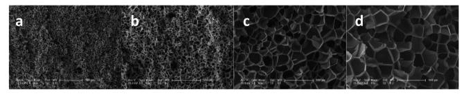
Fig. 10 SEM images of PEK-C (S2) foams prepared in different pressure release rate. The pressure release time are: (a) 1 s; (b) 9.8 s; (c) 28.5 s; and (d) 47.6 s (saturation pressure is 12 MPa and temperature is 290  $^{\circ}$ C) (scale bar 500  $\mu$ m).
