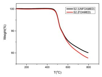
Fig. 7 TGA curves of S2 (before and after foamed at 280  $^{\circ}$ C and 12 MPa.) heated in N<sub>2</sub>.
