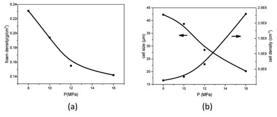
Fig. 9 Effect of foaming pressure on (a) foam density and (b) average cell size and cell density for PEK-C (S3) foams (foaming temperature: 280 °C).
