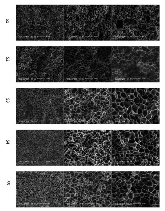
Fig. 2 SEM images of PEK-C foams with different gel contents (saturation time: 2 h; pressure: 12 MPa). The scale bar for S1 at 290  $^{\circ}$ C is 100  $\mu$ m, and the scale bar for the other samples is 50  $\mu$ m.
