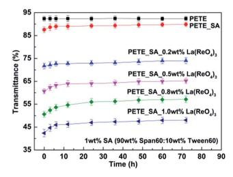
Fig. 4 Transmittances of PETE containing different concentrations of  $La(ReO_4)_3$  additive with the inclusion of SA.
