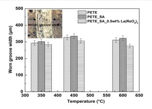
Fig. 10 Average width values of the worn track lubricated by different lubricating media.
