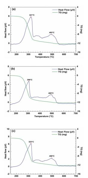
Fig. 5 DTA/TG curves of different lubricating samples: (a) PETE; (b) PETE\_SA; (c) PETE\_SA\_0.5 wt%  $La(ReO_4)_3$ .
