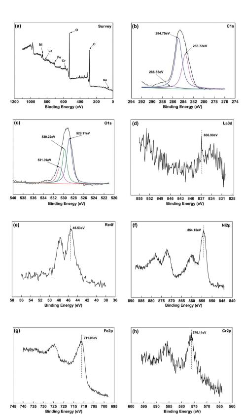
Fig. 12 XPS spectra of major elements on the worn surface of the superalloy disc lubricated by PETE containing 0.5 wt%  $La(ReO_4)_3$  after sliding test at 600 °C: (a) survey; (b) C1s; (c) O1s; (d) La3d; (e) Re4f; (f) Ni2p; (g) Fe2p; (h) Cr2p.
