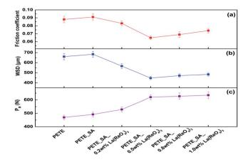
Fig. 6 Effect of different concentrations of  $La(ReO_4)_3$  additive on the average values of friction coefficient, wear scar diameter and maximum nonseizure load: (a) friction coefficient; (b) wear scar diameter; (c) maximum nonseizure load.
