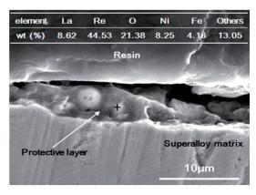
Fig. 13 Cross-section image of worn surface lubricated by PETE with 0.5 wt% La(ReO<sub>4</sub>)<sub>3</sub> after sliding test at 600 °C and EDS analysis of marked point.
