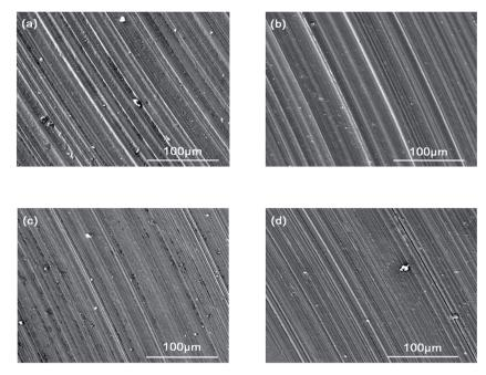
Fig. 7 SEM images of wear scars lubricated by different lubricating samples: (a) PETE\_SA; (c) PETE\_SA\_0.5 wt%  $La(ReO_4)_3$ ; (d) PETE\_SA\_1.0 wt%  $La(ReO_4)_3$ .
