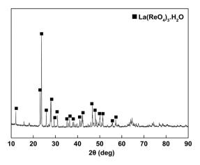
Fig. 2 XRD pattern of synthesized powder.
