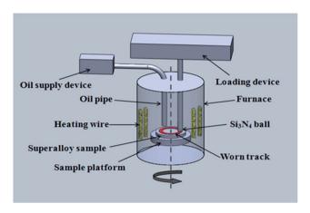
Fig. 1 Schematic illustration of UMT-2M ball-on-disc tribotester.
