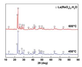
Fig. 11 XRD patterns of  $La(ReO_4)_3$  powder after heat treatment at different temperatures for 10 minutes.
