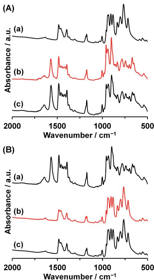
Fig. 4 (A) IR spectra of (a) **Mn2**, (b) **Mn2** treated with 1.0 equiv. of  $\text{Mn}(\text{OAc})_2$ , and (c) **Mn3**. (B) IR spectra of (a) **Mn3**, (b) **Mn3** treated with 5.0 equiv. of  $\{\text{Et}_4\text{N}\}[\text{VO}_3]$ , and (c) **Mn2**.
