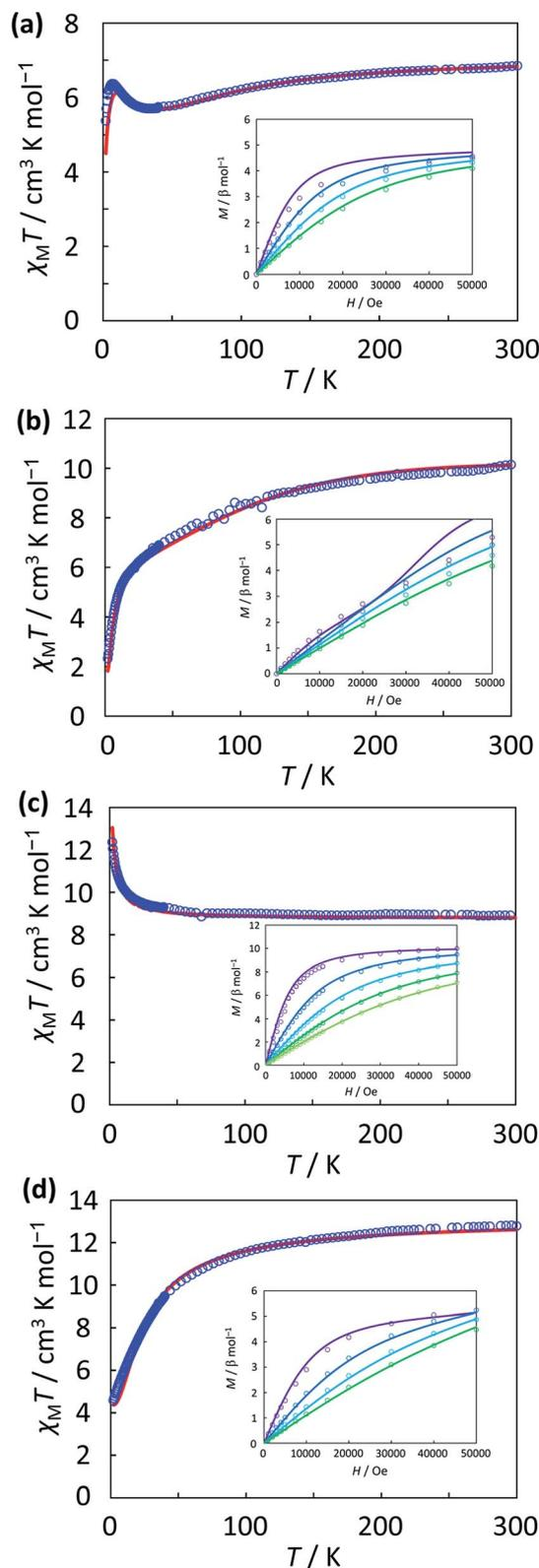
Fig. 6 Temperature dependence of  $\chi_M T$  values of (a) **Co2**, (b) **Co3**, (c) **Mn2**, and (d) **Mn3** in the temperature range of 2.0–300 K under 1000 Oe field. Inset represents the field dependence of magnetization data. Solid lines represent the fitting data.
