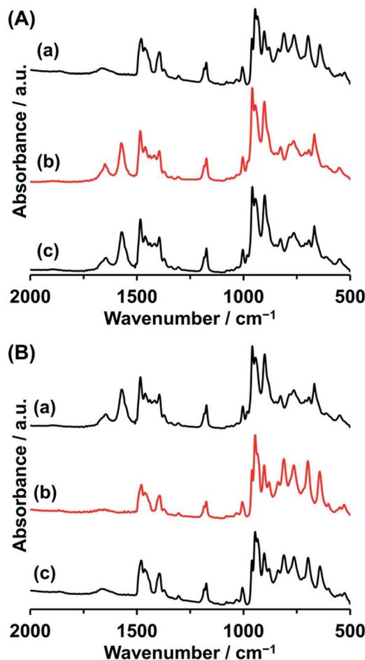
Fig. 2 (A) IR spectra of (a) Co2, (b) Co2 treated with 1.0 equiv. of Co(OAc)<sub>2</sub>, and (c) Co3. (B) IR spectra of (a) Co3, (b) Co3 treated with 5.0 equiv. of {Et<sub>4</sub>N}[VO<sub>3</sub>], and (c) Co2.
