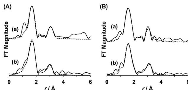
Fig. 5 Mn–K-edge Fourier transform of (A) **Mn2** (a) in propylene carbonate and (b) in BN pellets and (B) **Mn3** (a) in propylene carbonate and (b) in BN pellets. Experimental and simulated data are shown as solid and dotted lines, respectively.
