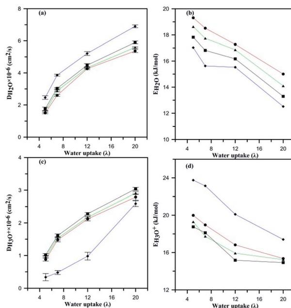
Fig. 9 Diffusion coefficients of (a) water molecules and (c) hydronium ions; activation energy of diffusion of (b) water molecules and (d) hydronium ions. (◆) undoped Nafion®, (●)  $\text{PW}^{3-}$ /Nafion®, (▲)  $\text{SiW}^{4-}$ /Nafion®, (■)  $\text{AlW}^{5-}$ /Nafion®.
