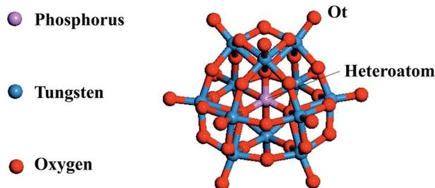
Fig. 1 The simulated  $\alpha$ -Keggin [PW<sub>12</sub>O<sub>40</sub>]<sup>3-</sup> anion and definition of terminal oxygen (OT).
