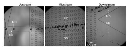
Fig. 4 Separation of the W/O main droplets from satellite droplets through a single-step DLD array.  $Q_c = 3.0$  mL  $h^{-1}$  and  $Q_d = 0.05$  mL  $h^{-1}$ .
