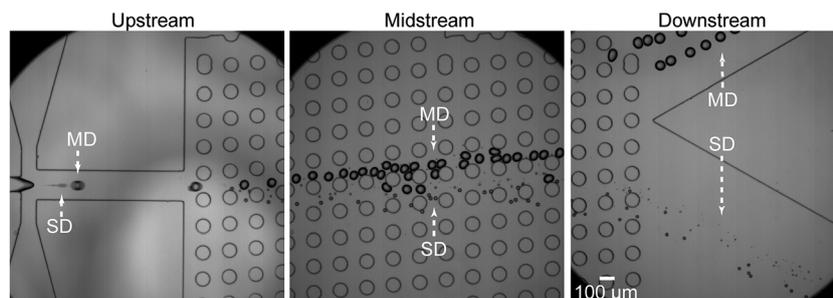
**Fig. 4** Separation of the W/O main droplets from satellite droplets through a single-step DLD array.  $Q_c = 3.0 \text{ mL h}^{-1}$  and  $Q_d = 0.05 \text{ mL h}^{-1}$ .
