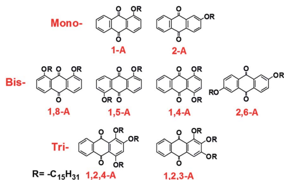
Scheme 1 Chemical structures of mono-, bis-, and tri-substituted anthraquinone derivatives.
