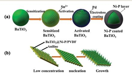
Fig. 1 Schematic illustration of (a) formation of Ni-P-coated BaTiO<sub>3</sub> and (b) formation of aligned PANI on the surface of the composites.
