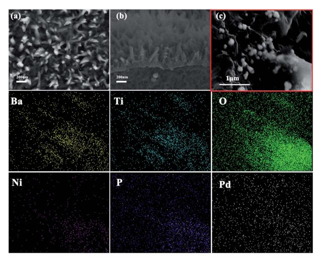
Fig. 4 SEM images of BaTiO<sub>3</sub>@Ni-P/PVDF/PANI: (a) surface image; (b) edge of the cross-sectional image; (c) middle of the cross-sectional image; and SEM-EDS elemental mappings that correspond to (c): Ba, Ti, O, Ni, P and Pd elements.
