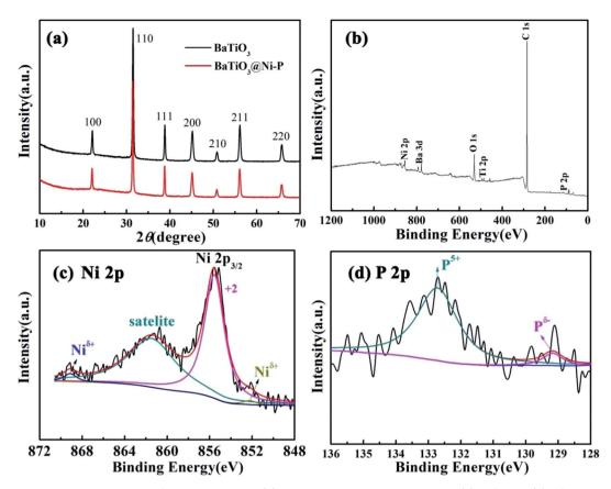
Fig. 3 (a) XRD patterns of the samples. XPS survey spectra of (b) wide scan, peak deconvolution of (c) Ni 2p and (d) P 2p for BaTiO<sub>3</sub>@Ni-P.
