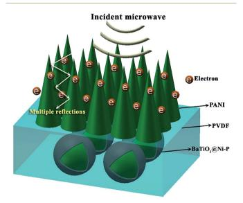
Fig. 8 Schematic illustration of the absorption mechanism of BaTiO<sub>3</sub>@Ni-P/PVDF/PANI.
