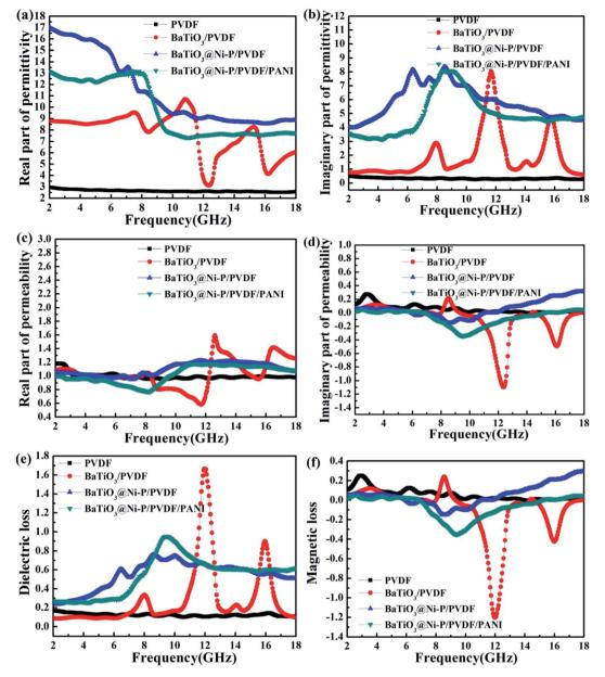
Fig. 5 Complex permittivity of samples: (a) real part and (b) imaginary part. Complex permeability of samples: (c) real part, (d) imaginary part, (e) dielectric loss, and (f) magnetic loss of samples.
