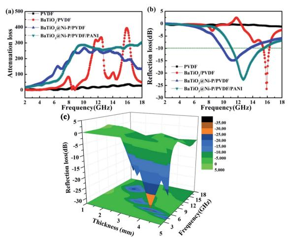
Fig. 7 (a) Attenuation constant  $\alpha$  of the samples, (b) reflection loss of the samples with a thickness of 2 mm, and (c) reflection loss of BaTiO<sub>3</sub>@Ni-P/PVDF/PANI with different thickness.
