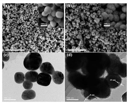
Fig. 2 SEM images of (a) pristine BaTiO<sub>3</sub> and (b) BaTiO<sub>3</sub>@Ni-P. TEM images of (c) pristine BaTiO<sub>3</sub> and (d) BaTiO<sub>3</sub>@Ni-P.
