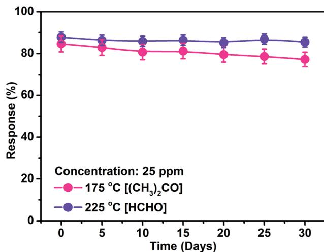
**Fig. 9** Life-time performances of nanocube  $\text{In}_2\text{O}_3$ @RGO heterostructure based gas sensor functioned at 175 °C and 225 °C for 25 ppm concentration to acetone and formaldehyde, respectively.
