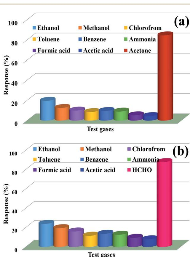
Fig. 8 Selectivity profiles for 25 ppm concentration of acetone (a) and formaldehyde (b) at optimum working temperature 175 °C and 225 °C, respectively, based on nanocube  $\text{In}_2\text{O}_3@\text{RGO}$  heterostructure gas sensor.
