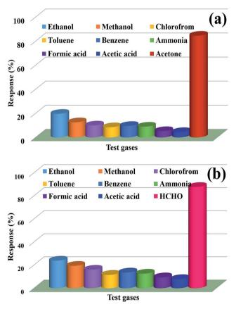
Fig. 8 Selectivity profiles for 25 ppm concentration of acetone (a) and formaldehyde (b) at optimum working temperature 175  $^{\circ}$ C and 225  $^{\circ}$ C, respectively, based on nanocube  $In_2O_3$ @RGO heterostructure gas sensor.
