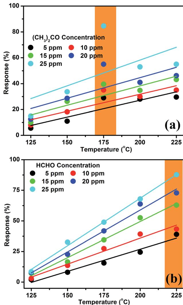
Fig. 4 Response characteristics of acetone (a) and formaldehyde (b) based on the nanocube  $\text{In}_2\text{O}_3@\text{RGO}$  heterostructure sensor as a function of operating temperature for distinct test gas concentrations.
