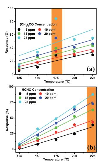
Fig. 4 Response characteristics of acetone (a) and formaldehyde (b) based on the nanocube  $In_2O_3$ @RGO heterostructure sensor as a function of operating temperature for distinct test gas concentrations
