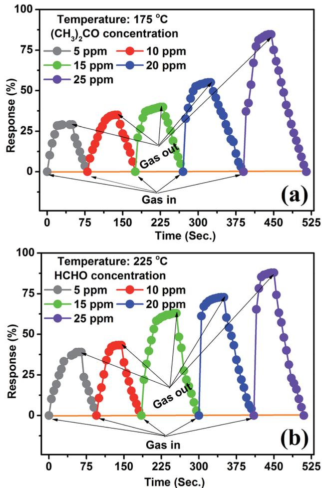
Fig. 6 The response/recovery real time profiles of the nanocube  $\text{In}_2\text{O}_3@\text{RGO}$  heterostructure based gas sensor to acetone (a) and formaldehyde (b) for 5–25 ppm concentration at optimum working temperature 175 °C and 225 °C, respectively.
