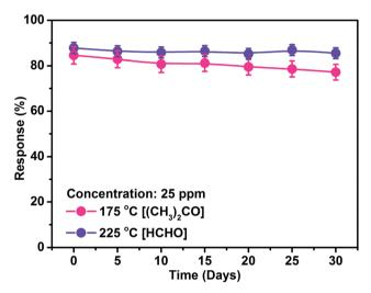
Fig. 9 Life-time performances of nanocube  $In_2O_3$ @RGO heterostructure based gas sensor functioned at 175 °C and 225 °C for 25 ppm concentration to acetone and formaldehyde, respectively.
