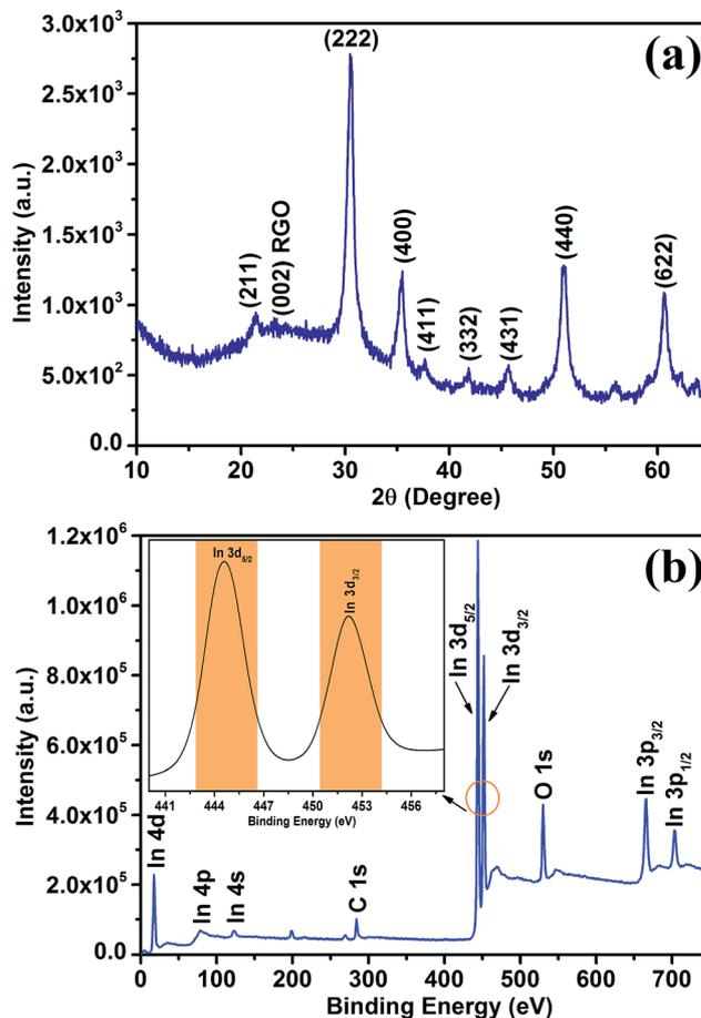
Fig. 1 Typical XRD pattern (a) and XPS spectrum (b) of as obtained nanocube  $\text{In}_2\text{O}_3$ @RGO heterostructure (inset in (b) depicts the convoluted characteristic peaks of In 3d).
