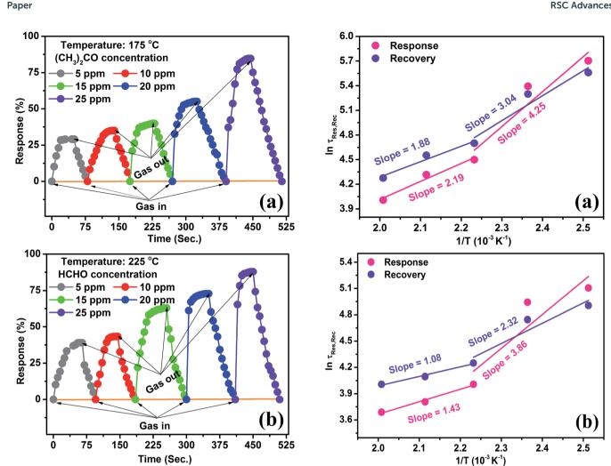
Fig. 6 The response/recovery real time profiles of the nanocube In<sub>2</sub>O<sub>3</sub>@RGO heterostructure based gas sensor to acetone (a) and formaldehyde (b) for 5-25 ppm concentration at optimum working temperature 175 °C and 225 °C, respectively.
