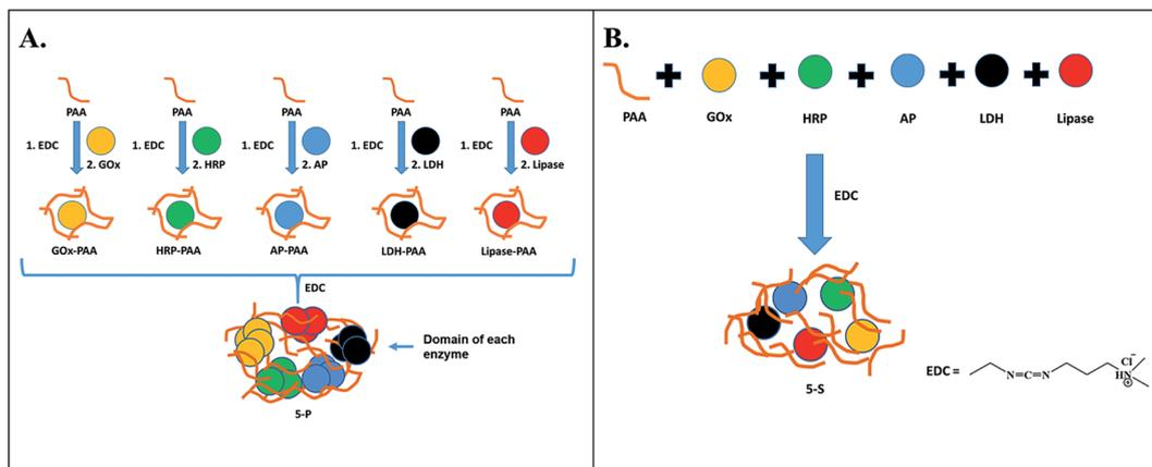
**Scheme 1** Two different routes to synthesize MECs. In Route 1 (A), individual enzyme–PAA conjugates are synthesized using EDC chemistry, and then further crosslinked to prepare 5-P. In Route 2 (B), PAA and all 5 enzymes are mixed together and subsequently crosslinked using EDC to prepare 5-S. Here, GOx, HRP, AP, LDH and Lip are represented by yellow, green, blue, black and red circles, respectively, and PAA is shown as brown strings.
