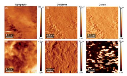
Fig. 4 Micrographs of 1 vol% undoped CNT/PVDF nanocomposite biased at 4 V before (a-c) and after (d-f) chemical etching.
