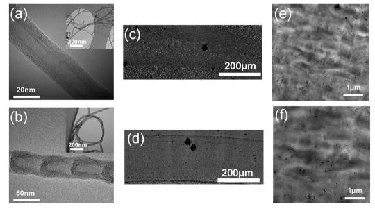
Fig. 2 (a and b) Transmission electron micrographs of (a) undoped CNT and (b) N-doped CNT, with inset showing overall structure at lower magnification; (c and d) optical and (e and f) transmission electron micrographs of undoped CNT/PVDF (c and e) and N-doped CNT/PVDF (d and f) nanocomposites, showing the 2D dispersion state and agglomeration state.
