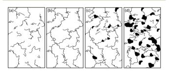
Fig. 3 Possible CNT dispersion state in the nanocomposite. Nanofiller dispersion (a) below percolation threshold, (b) above percolation threshold and with minimal agglomeration, (d) above percolation threshold and significant agglomeration.
