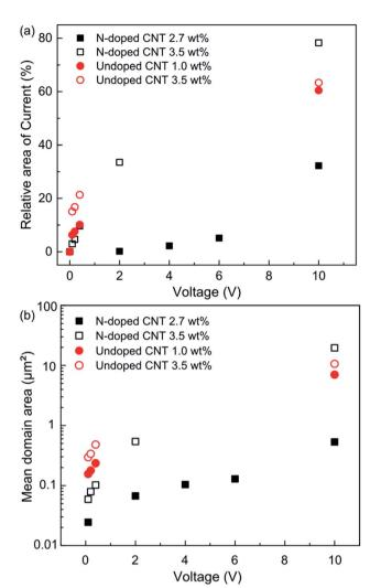
Fig. 10 (a) The percentage area (relative) of current observed per area scanned ( $A_t$ ) and (b) the mean domain areas calculated for both N-doped (black filled/open squares) and undoped (red filled/open circles) CNT/PVDF nanocomposite samples. Filled squares/circles contain lower wt% CNTs, while open squares/circles contain 3.5 wt% CNTs.
