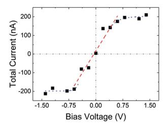
Fig. 7 Representative I-V curve from 3.5 vol% undoped CNT/PVDF sample. Y-axis is the total current measured over  $40 \times 40 \ \mu m^2$  scan area. The blue dotted and red dashed line are for guidance only, but highlight the region influenced by the linear resistance of the composite (red dashed line) and saturation of the amplifier (blue dotted line). A grey dashed line demarks the values of 0 V and 0 nA.
