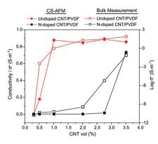
Fig. 11 Macro and nanoscopic conductivity values of N-doped (squares) and undoped (dots) CNT/PVDF nanocomposites for different CNT concentration. Conductivity values obtained by CS-AFM method is shown in left side *Y*-axis (closed symbols), and that of bulk measurements in right side *Y*-axis (open symbols). The connecting lines are for guidance. Scan area was  $40 \times 40 \ \mu m^2$  for all samples.
