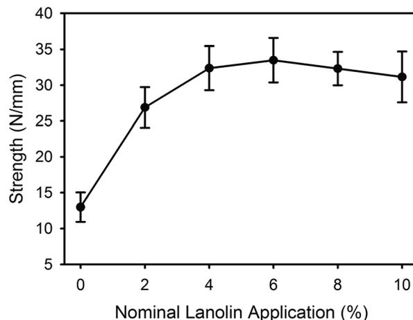
Fig. 6 Tear strength of leather with lanolin content.
