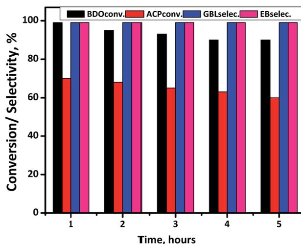
Fig. 11 Time-on-stream study for coupling of ACP hydrogenation and BDO dehydrogenation over Cu/SiO<sub>2</sub> catalyst at 523 K for 5 h. Reaction conditions: catalyst = 0.5 g, T = 523 K, WHSV = 2 h<sup>-1</sup>, ACP/BDO mole ratio = 1 : 2, feed = 1 mL h<sup>-1</sup> and N<sub>2</sub> flow = 18 mL min<sup>-1</sup>.
