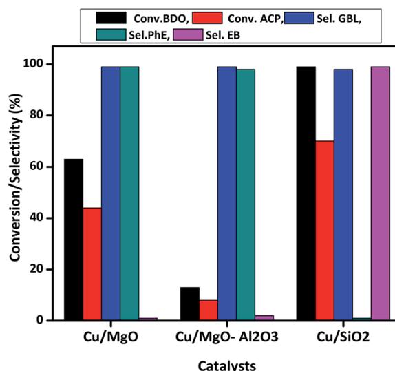
Fig. 9 Coupling of ACP hydrogenation and BDO dehydrogenation over supported copper catalysts at 523 K. Reaction conditions: catalyst = 0.5 g, WHSV = 2  $\text{h}^{-1}$ , ACP and BDO mole ratio = 1 : 2, feed flow = 1  $\text{mL h}^{-1}$  and  $\text{N}_2$  flow = 18  $\text{mL min}^{-1}$ .
