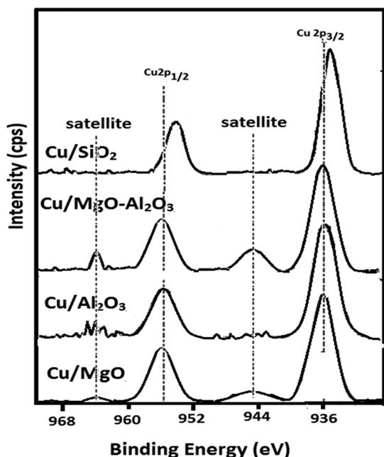
Fig. 6 XPS patterns of Cu of supported copper catalysts.
