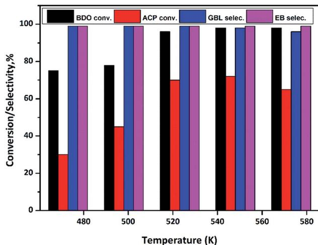
Fig. 10 Effect of temperatures on coupling of BDO dehydrogenation and ACP hydrogenation over Cu/SiO<sub>2</sub> catalyst. Reaction conditions: catalyst = 0.5 g, WHSV = 2 h<sup>-1</sup>, temperature = 473–573 K, ACP and BDO mole ratio = 1 : 2, feed flow = 1 mL h<sup>-1</sup> and N<sub>2</sub> flow = 18 mL min<sup>-1</sup>.
