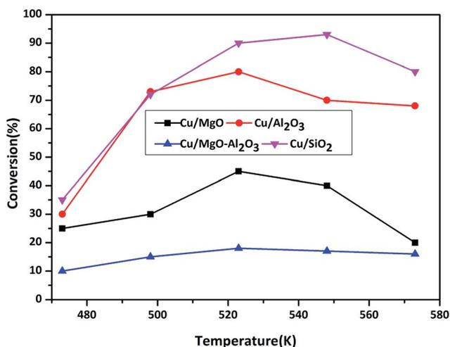
Fig. 8 ACP transformation as a function of temperature over supported copper catalysts. Reaction conditions: catalyst = 0.5 g, WHSV = 2  $\text{h}^{-1}$ , ACP and BDO mole ratio = 1 : 2, feed flow = 1  $\text{mL h}^{-1}$  and  $\text{H}_2$  gas flow = 18  $\text{mL min}^{-1}$ .
