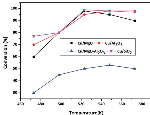
Fig. 7 Conversion of BDO as a function of temperature over different copper catalysts. Reaction conditions: catalyst = 0.5 g, WHSV = 2 h<sup>-1</sup>, BDO feed flow = 1 mL h<sup>-1</sup> and N<sub>2</sub> gas flow = 18 mL min<sup>-1</sup>.
