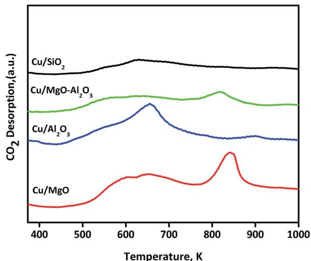
Fig. 5 CO<sub>2</sub>-TPD patterns of various supported copper catalysts.
