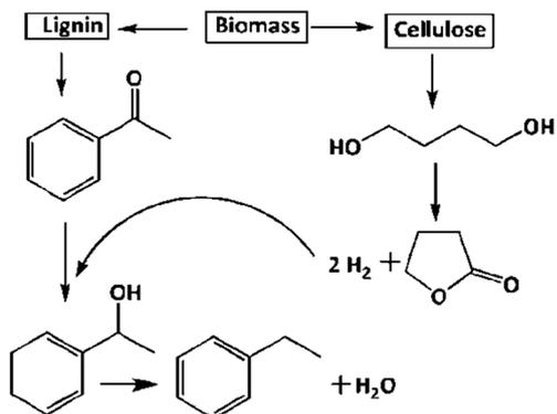
Scheme 1 Reductive upgrading of acetophenone (ACP) to ethylbenzene (EB) and 1,4-butanediol (BDO) to  $\gamma$ -butyrolactone (GBL) via coupling of simultaneous hydrogenation and dehydrogenation process.
