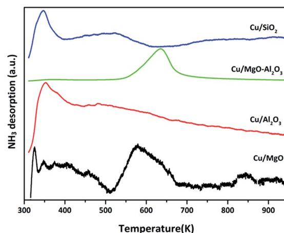
Fig. 4 NH<sub>3</sub>-TPD patterns of various supported copper catalysts.
