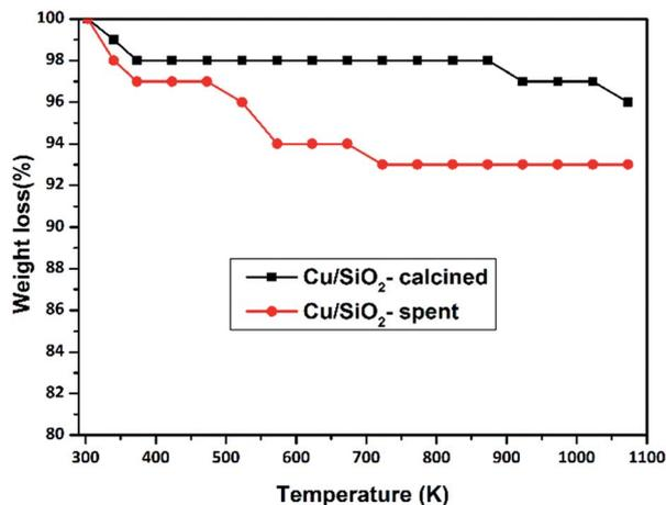
Fig. 12 TGA analysis of calcined and spent Cu/SiO<sub>2</sub> catalysts.
