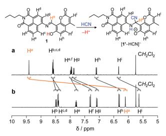
Fig. 3  $^{-1}$ H NMR chart of 1 (10 mM) measured (a) without and (b) with 1 equiv. of CN $^{-}$  (400 MHz, 30  $^{\circ}$ C, DMSO-d<sub>6</sub>).
