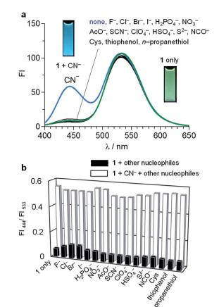
Fig. 1 (a) Fluorescence spectra ( $\lambda_{ex}=385$  nm) of 1 (10  $\mu$ M) with 200 equiv. of each nucleophile in a buffered water/MeCN mixture (1/1 v/v; HEPES 0.1 M, pH 7.0) at 25 °C. (b) Intensity obtained (black) with 200 equiv. of each nucleophile and (white) 200 equiv. of CN $^-$  and other nucleophiles.
