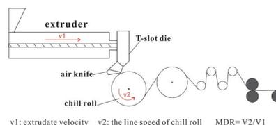
Fig. 1 The schematic for processing cast films.
