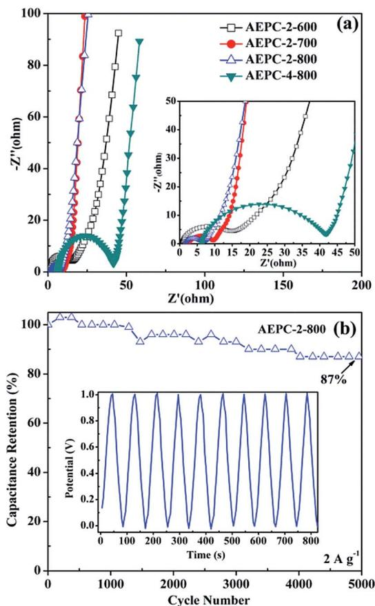
Fig. 7 (a) Nyquist plots of four carbon capacitors and inset is the enlarged view of high-frequency region, (b) the cycling performance of AEPC-2-800 capacitor at  $2 \text{ A g}^{-1}$  and inset shows the first 10 cycles.
