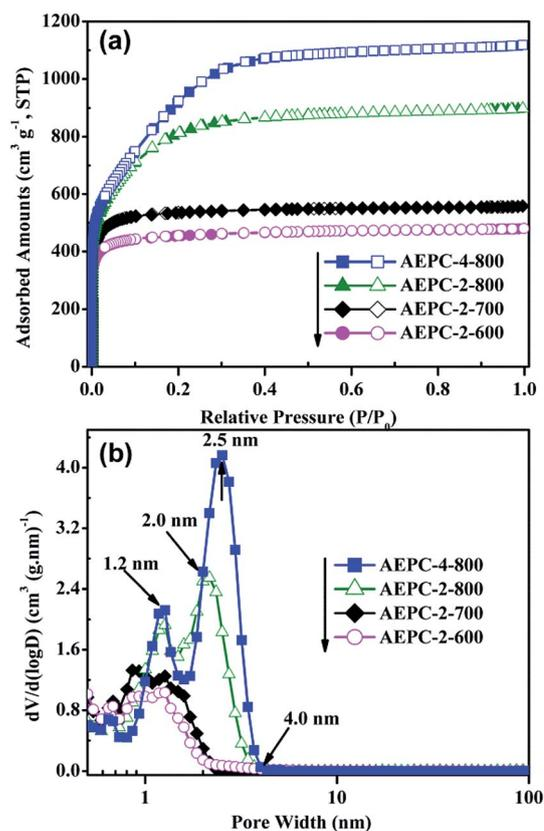
Fig. 2 (a)  $\text{N}_2$  sorption isotherms for carbons at  $-196^\circ\text{C}$ , and (b) corresponding pore size distributions.
