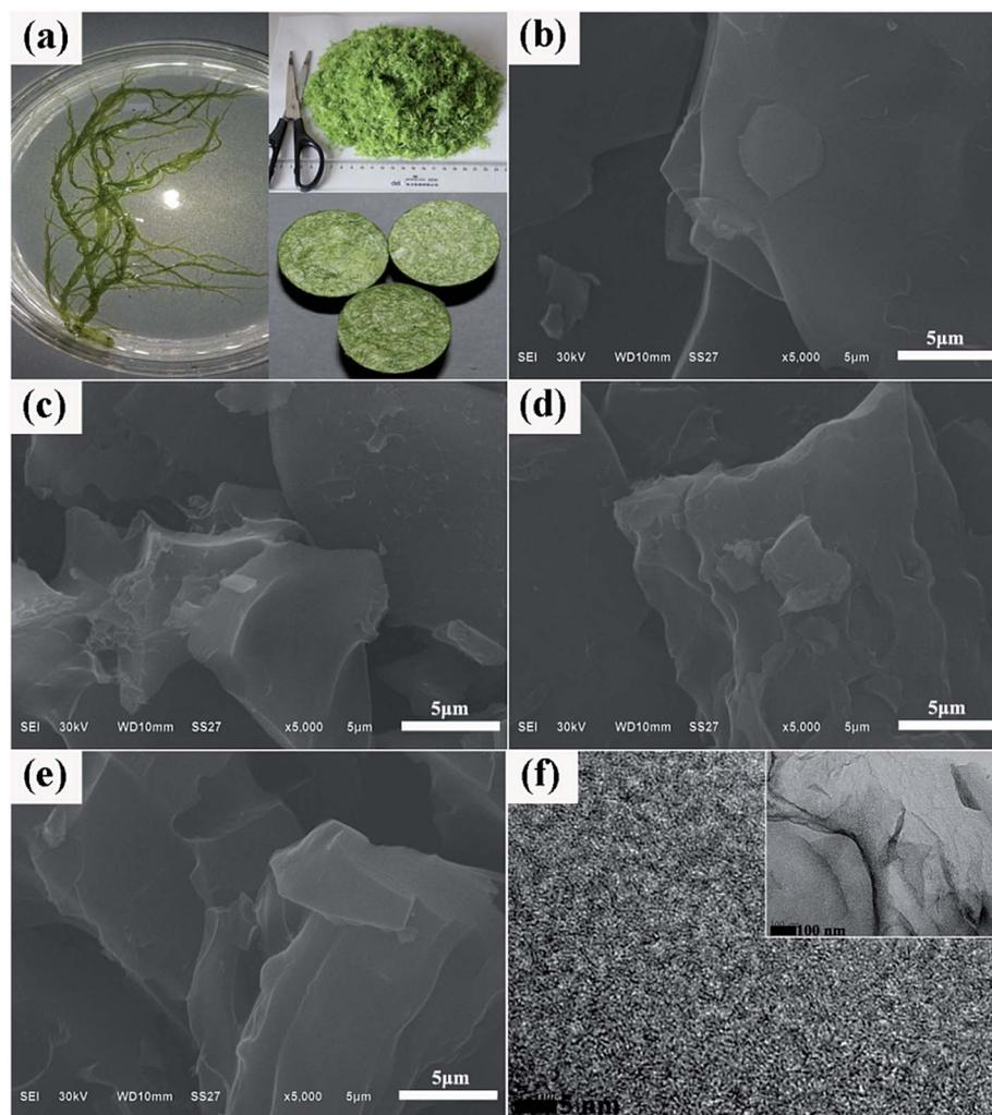
Fig. 1 (a) Photos for fresh EP; SEM images for (b) AEPC-2-600, (c) AEPC-2-700, (d) AEPC-2-800, and (e) AEPC-4-800; representative TEM images for (f) AEPC-4-800.
