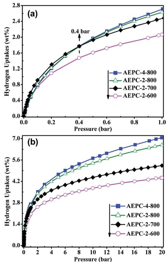
Fig. 5 H<sub>2</sub> adsorption isotherms at −196 °C for the carbons at (a) 1 bar, and (b) 20 bar.
