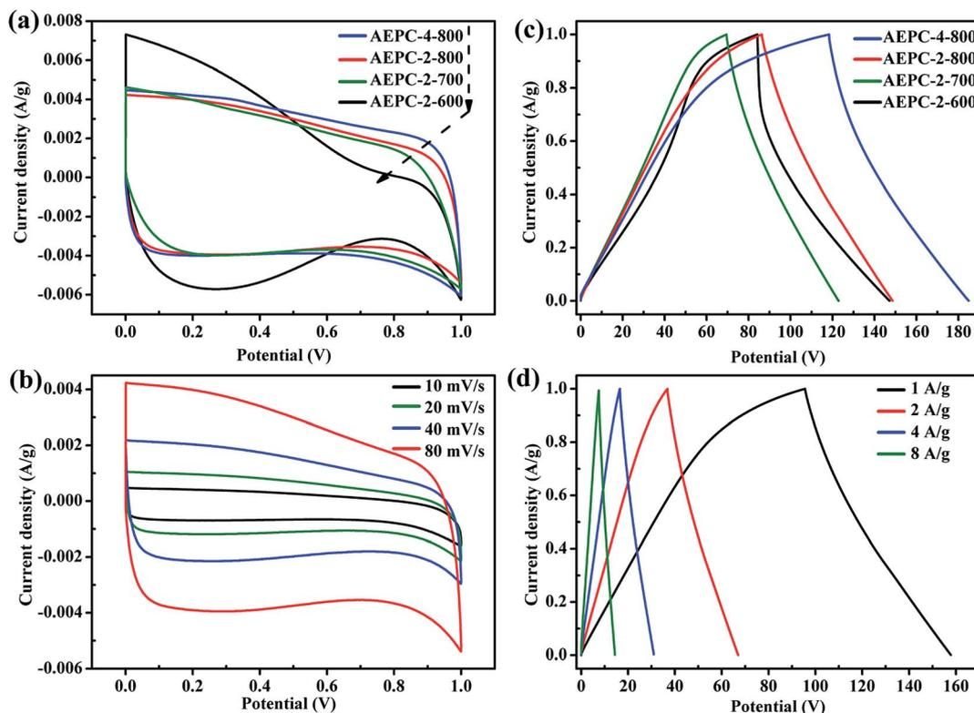
Fig. 6 (a) CV curves at  $80 \text{ mV s}^{-1}$ , (b) CV curves of AEPC-2-800 capacitor at various scan rates, (c) GCD curves at  $1 \text{ A g}^{-1}$ , (d) GCD curves of AEPC-2-800 capacitor at various current densities.
