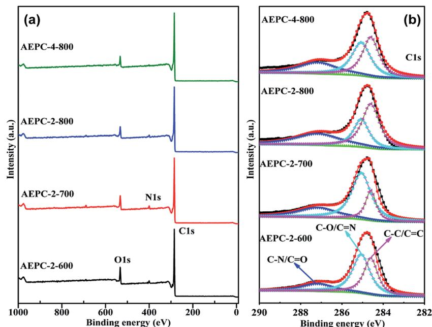
Fig. 3 The XPS survey spectra and high-resolution C1s region of the activated carbons.
