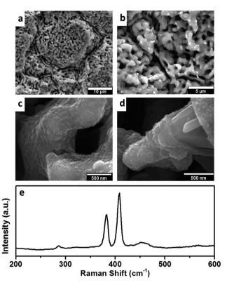
Fig. 3 (a-c) Scanning electron micrographs of MoS<sub>2</sub> covered 3D stainless steel-graphene structures. A highly conformal coating on the surface is achieved by electrodeposition technique. The porous nature of the current collector is preserved with no clogging or large particulates; (d) an isolated defect in the electrodeposition, shown to highlight the thickness of the MoS<sub>2</sub> layer; (e) Raman spectrum of the structure wherein the bands correspond to MoS<sub>2</sub>.
