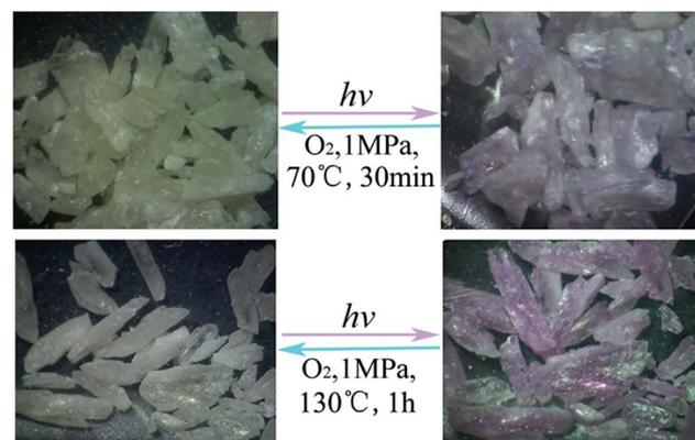
Fig. 3 Photochromism of **1** (top) and **2** (bottom).
