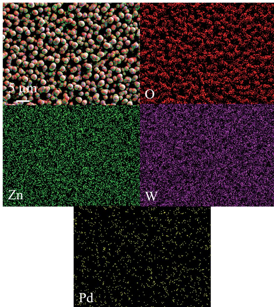
Fig. 3 Elemental mapping of surface images of Pd/WO<sub>3</sub>-ZnO thin film.
