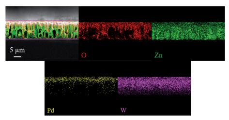
Fig. 4 Elemental mapping of cross sectional images of Pd/WO<sub>3</sub>-ZnO thin film.
