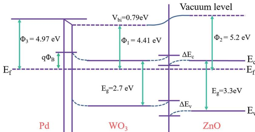
Fig. 8 The energy banding diagram of the Pd/WO<sub>3</sub>-ZnO sensor which establish the bending of the band after the equalization of the Fermi levels.
