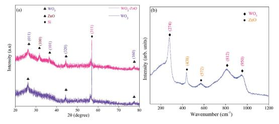
Fig. 1 (a) XRD spectra of WO<sub>3</sub> and Pd/WO<sub>3</sub>-ZnO thin films, and (b) Raman spectra of Pd/WO<sub>3</sub>-ZnO thin films.
