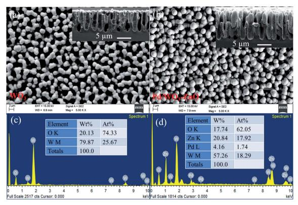
Fig. 2 (a and b) FE-SEM images with corresponding cross section images, and (c and d) EDS spectra of  $WO_3$  and  $Pd/WO_3$ –ZnO thin films, respectively.
