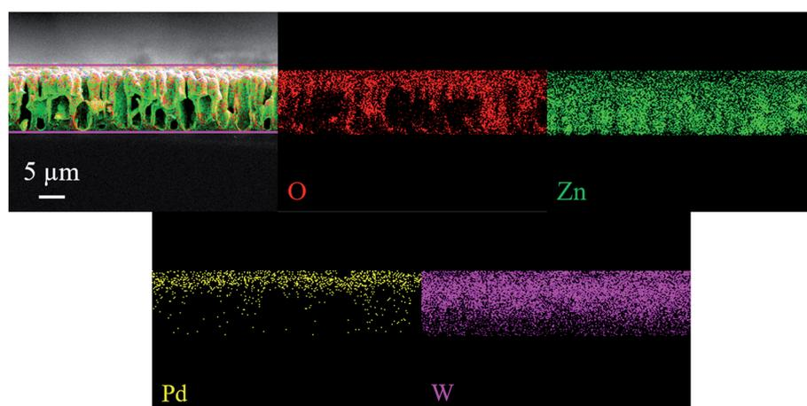
Fig. 4 Elemental mapping of cross sectional images of Pd/WO<sub>3</sub>-ZnO thin film.
