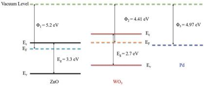
Fig. 7 Energy band diagram of Pd/WO<sub>3</sub>-ZnO thin film sensor before thermal equilibrium.
