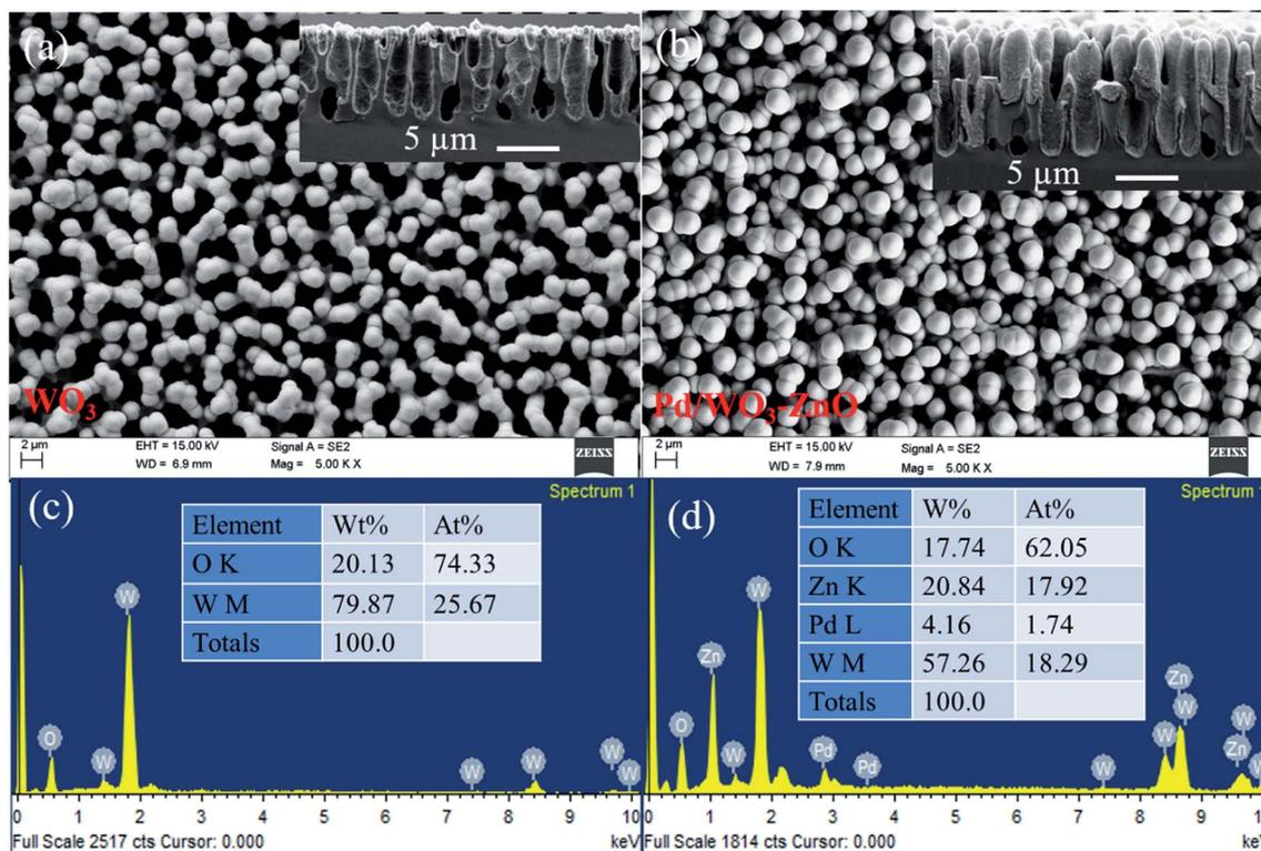
Fig. 2 (a and b) FE-SEM images with corresponding cross section images, and (c and d) EDS spectra of WO<sub>3</sub> and Pd/WO<sub>3</sub>-ZnO thin films, respectively.
