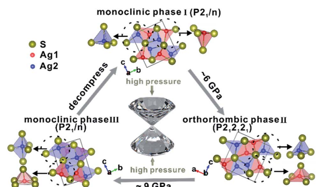
Fig. 4 Schematic structures of the phase I, II, and III unit cells of the \text{Ag}_2\text{S} compounds. The pressures of the phase transitions during compression and decompression sequences are also indicated.
