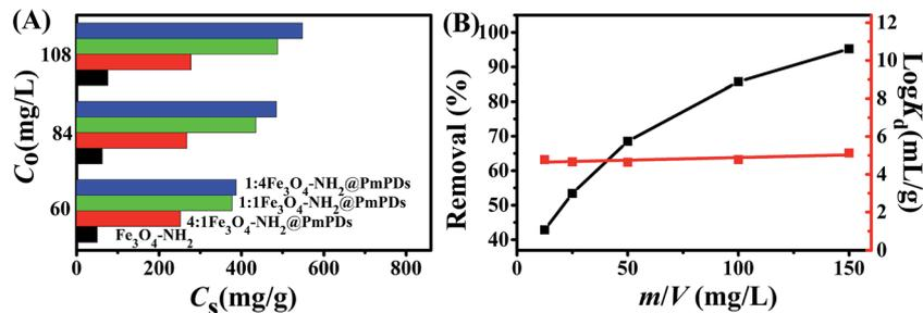
Fig. 3 Adsorbents with different mass ratios for Cr(vi) removal (A); the adsorption of Cr(vi) on 1 : 1Fe<sub>3</sub>O<sub>4</sub>-NH<sub>2</sub>@PmPDs as a function of adsorbent content (B).  $m/V = 0.15 \text{ g L}^{-1}$ , time = 12 h.  $[\text{Cr(vi)}] = 60 \text{ mg L}^{-1}$ .
