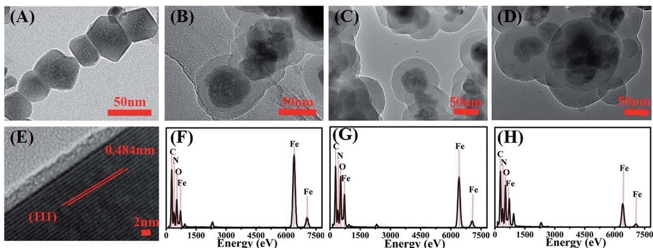
Fig. 1 Representative TEM, HRTEM, and EDS images.  $\text{Fe}_3\text{O}_4\text{-NH}_2$  (A and E), 4 : 1 $\text{Fe}_3\text{O}_4\text{-NH}_2\text{@PmPDs}$  (B and F), 1 : 1 $\text{Fe}_3\text{O}_4\text{-NH}_2\text{@PmPDs}$  (C and G), and 1 : 4 $\text{Fe}_3\text{O}_4\text{-NH}_2\text{@PmPDs}$  (D and H).
