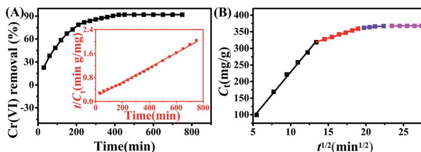
**Fig. 6** The effect of contact time on adsorption capacity of 1 : 1Fe<sub>3</sub>O<sub>4</sub>-NH<sub>2</sub>@PmPDs and fitting of the pseudo-second-order kinetic model (A) and intraparticle diffusion model (B).  $m/V = 0.15$  g L<sup>-1</sup>, [Cr(vi)] = 60 mg L<sup>-1</sup>.
