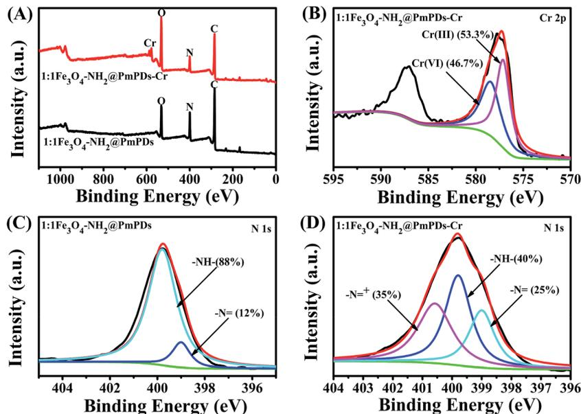
Fig. 7 XPS wide spectra of 1 : 1Fe<sub>3</sub>O<sub>4</sub>-NH<sub>2</sub>@PmPDs before and after Cr(vi) adsorption (A), Cr 2p (B), N 1s XPS spectra of 1 : 1Fe<sub>3</sub>O<sub>4</sub>-NH<sub>2</sub>@PmPDs (C) and 1 : 1Fe<sub>3</sub>O<sub>4</sub>-NH<sub>2</sub>@PmPDs with Cr(vi) adsorbed (D).
