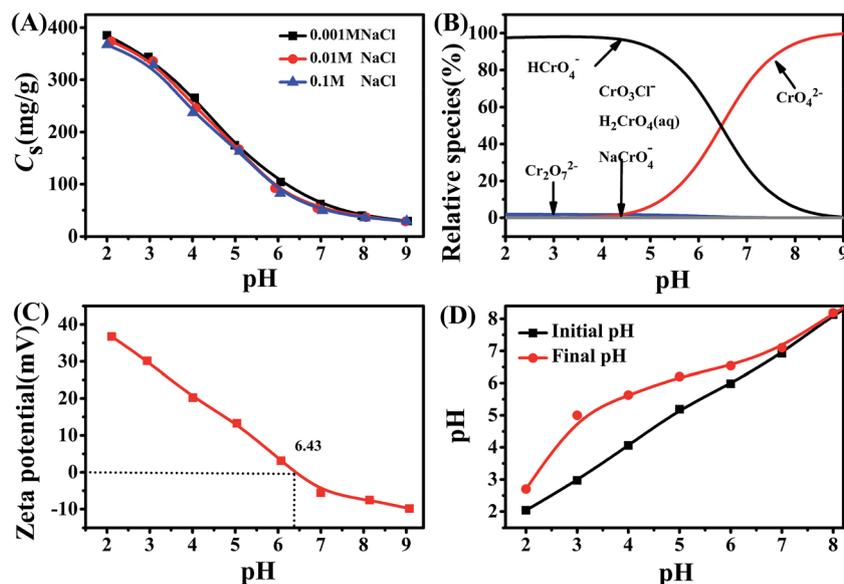
Fig. 4 Effect of pH on Cr(VI) adsorption on 1 : 1Fe<sub>3</sub>O<sub>4</sub>-NH<sub>2</sub>@PmPDs at different ionic strengths (A); distribution of Cr(VI) species in aqueous solutions (B); zeta potentials of 1 : 1Fe<sub>3</sub>O<sub>4</sub>-NH<sub>2</sub>@PmPDs at various solution pH values (C); and the change of initial pH and final pH (D).  $m/V = 0.15 \text{ g L}^{-1}$ , time = 12 h,  $[\text{Cr(VI)}] = 60 \text{ mg L}^{-1}$ .
