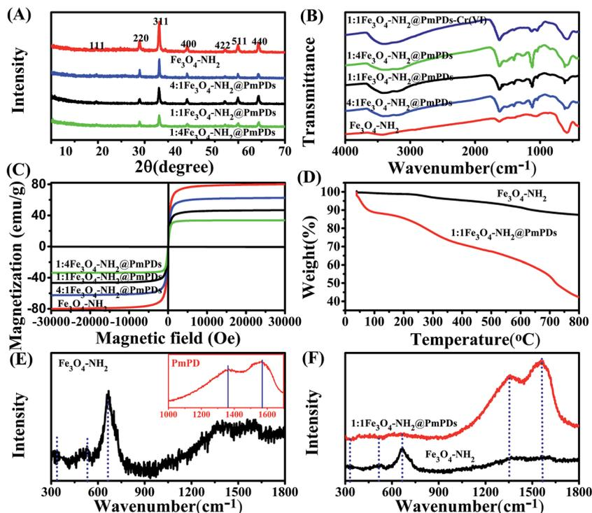
Fig. 2 XRD patterns (A), FT-IR spectra (B), magnetic hysteresis loop (C), TGA (D), and Raman spectra (E and F) of  $\text{Fe}_3\text{O}_4\text{-NH}_2$  and  $1:1\text{Fe}_3\text{O}_4\text{-NH}_2\text{@PmPDs}$ .
