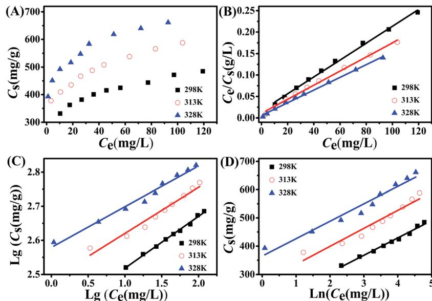
Fig. 5 The adsorption isotherms of Cr(vi) on 1 : 1Fe<sub>3</sub>O<sub>4</sub>-NH<sub>2</sub>@PmPDs (A) and the simulations with Langmuir (B), Freundlich (C), and Temkin (D) models at three different temperatures.  $m/V = 0.15 \text{ g L}^{-1}$ , time = 12 h.
