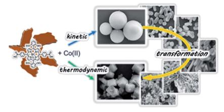
Fig. 5 A series of narrowly dispersed nano- and micro-sized CPs prepared from a Mn(III)-Pp metalloligand acid and Co(OAc)<sub>2</sub>, which morphologies diversified from amorphous spheres to crystalline cubes by varying reaction periods. [Reproduced from ref. 85 with permission from The Royal Society of Chemistry.]
