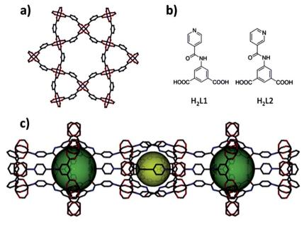
Fig. 11 (a) Layer segment of a kgm-MOF. (b) (Left) 5-(Isonicotinamido)isophthalic acid ( $H_2L^1$ ) and right: 5-(nicotinamido)isophthalic acid ( $H_2L^2$ ). (c) Hourglass-shaped channels with two primary types of cavities. C – gray, O – red, N – blue, Cu – plum. [Reproduced from ref. 119 with permission from The Royal Society of Chemistry.]
