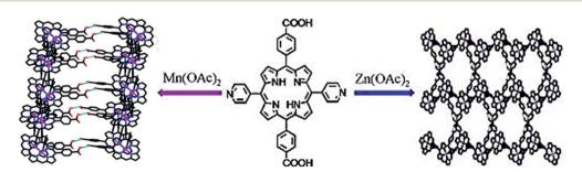
Scheme 17 CPs obtained by the interaction of Mn(|||) and Zn(|||) acetates with 5,15-bis(4-carboxyphenyl)-10,20-dipyridyl-Pp. [Reprinted from ref. 216. Copyright 2014, with permission from Elsevier.]
