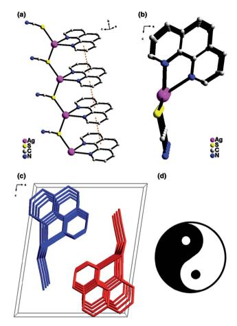
Fig. 17 (a) Diagram of the asymmetric chain in CP exhibiting strong  $\pi$ - $\pi$  interactions among the phen rings (orange dash lines). (b) Perspective view of the chain along the b direction. (c) The unit cell packing structure of CP along the b direction. (d) The patterning of T in Ji. [Reprinted from ref. 204. Copyright 2016, with permission from Springer.]
