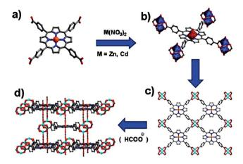
Fig. 3 (a) Deprotonated Mn-Pp ligand, (b) view of the coordination mode of Mn-Pp and the coordination environments of M' and Mn atoms, (c) lamellar network of Mn-Pp linking up  $M'_2(COO)_4$  paddlewheel SBUs, (d) perspective view of the 3D Pp framework. Color codes: M', cyan or light-blue square pyramids; Mn, orange; O, red; N, blue; C, gray. [Reprinted with permission from ref. 81. Copyright 2013, American Chemical Society.]
