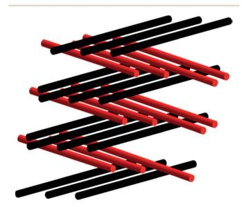
Fig. 14 Representation of cross-like arrangement of 1D chains in ABAB fashion to generate 3D plywood-like array in CP. [Reprinted with permission from ref. 144. Copyright 2016, American Chemical Society.]
