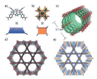
Fig. 1 The crystal structure and underlying network topology of PCN-222(Fe). The Fe-L¹ (a; blue square) is connected to four 8-connected Zr $_6$  clusters (b; light orange cuboid), generating a 3D network with Kagome-like topology (d, e) and large 1D channels (c; green pillar). Zr: black spheres, C: gray, O: red, N: blue, and Fe: orange. [Reprinted with permission from ref. 56. Copyright 2012, Wiley-VCH Verlag GmbH & Co. KGaA, Weinheim.]
