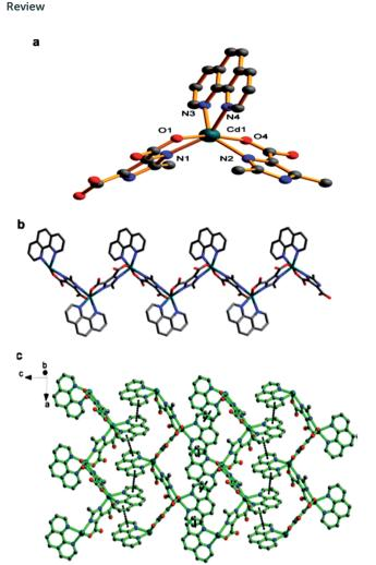
Fig. 15 (a) Molecular square structure of CP with [Cd(HL)(phen)] $_n$  unit based on 2-ethyl-1H-imidazole-4,5-dicarboxylic acid. (b) 1D chain of CP. (c) 2D sheet of CP supported by  $\pi-\pi$  stacking interactions. [Reprinted from ref. 158 Copyright 2012, with permission from Elsevier.]
