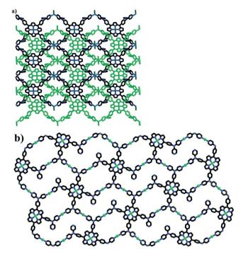
Fig. 20 (a) The interpenetrated 2D coordination networks constructed by Pp and MnCl<sub>2</sub>. (b) The 2D network composed of 50- and 70-membered metallomacrocycles, constructed from Pp and Cu(OAc)<sub>2</sub>. [Reprinted with permission from ref. 215. Copyright 2013, American Chemical Society.]
