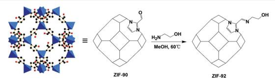
Fig. 24 Crystal structure of ZIF-90 and the covalent postsynthetic functionalization of aldehyde groups with ethanolamine to give ZIF-92. Color scheme: for C atoms, black; for N atoms, green; for O atoms, red. [Reprinted with permission from ref. 260. Copyright 2017, American Chemical Society.]
