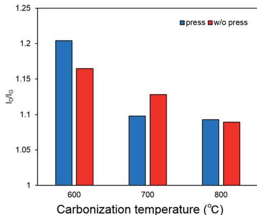
Fig. 4 Raman spectra of self-standing iron oxide/carbon composite electrospun nanofibers; (red) carbonization at 600, 700, and 800 °C without press treatment; (blue) carbonization at 600, 700, and 800 °C with press treatment.
