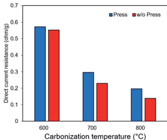
Fig. 8 Direct current resistance of self-standing iron oxide/carbon composite electrospun nanofibers: carbonization at 600, 700, and 800 °C with and without press treatment.
