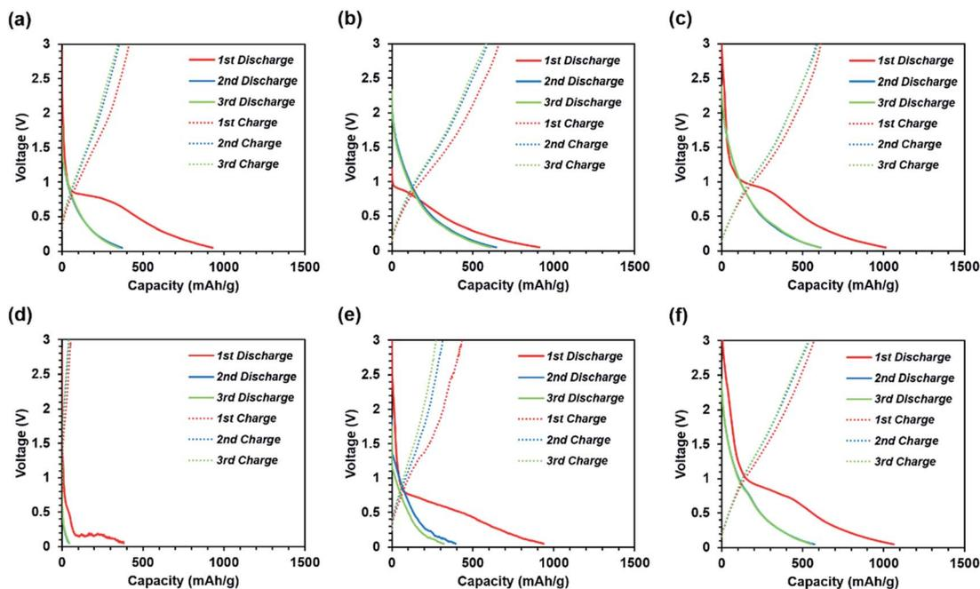
Fig. 5 1<sup>st</sup> to 3<sup>rd</sup> charge–discharge curves of self-standing iron oxide/carbon composite electrospun nanofibers at 100  $\text{mA g}^{-1}$ ; (a) carbonization at 600 °C, without press treatment; (b) carbonization at 700 °C, without press treatment; (c) carbonization at 800 °C, without press treatment; (d) carbonization at 600 °C, with press treatment; (e) carbonization at 700 °C, with press treatment; and (f) carbonization at 800 °C, with press treatment.
