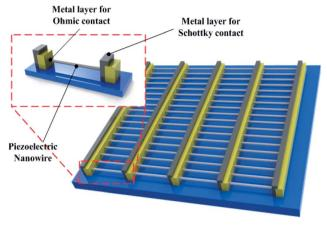
Fig. 4 Basic structure of LING
