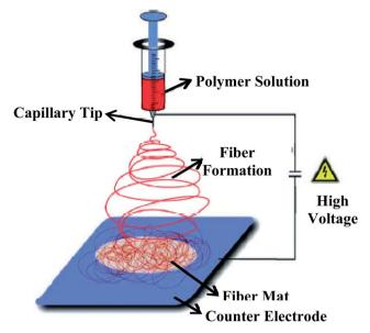
Fia. 12 Schematic illustration of a typical laboratory setup for conventional electrospinning with vertical feeding of the solution.90
