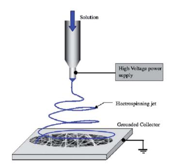
Fig. 13 Typical setup for electrospinning using a grounded collector.91
