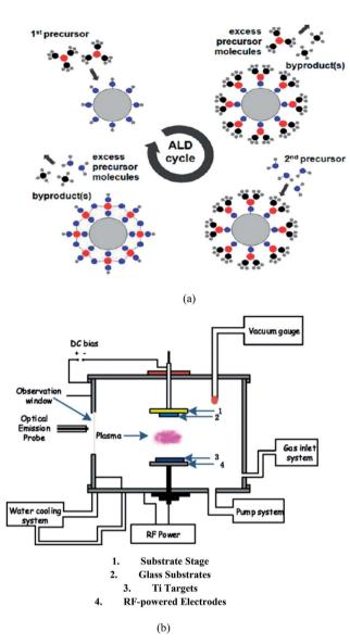
Fig. 11 Schematic representation of various seeding methods: (a) ALD83 and (b) RF magnetron sputtering.84
