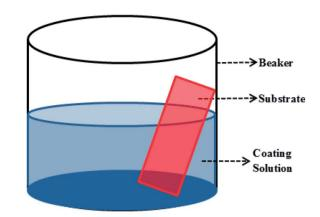
Fig. 14 Schematic of dip coating technique.
