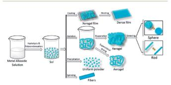
Fig. 9 Schematic illustration of sol-gel processes. 75
