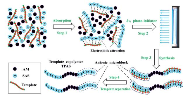
Fig. 8 The mechanism of template copolymerization.
