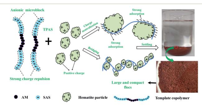
Fig. 13 Possible flocculation mechanism of the TPAS
