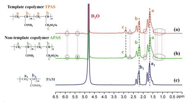
Fig. 5 <sup>1</sup>H NMR spectra of (a) TPAS, (a) APAS and (c) PAM
