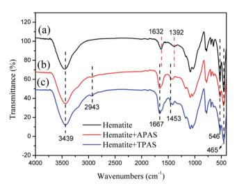
Fig. 12 FRIR spectra of hematite and flocs
