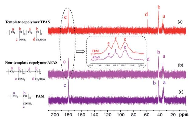
Fig. 6 <sup>13</sup>C NMR spectra of (a) TPAS, (a) APAS and (c) PAM.
