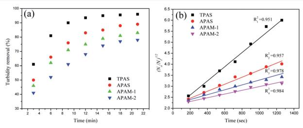
Fig. 11 The variation of turbidity removal (a) and (b)  $(N_0/N_0)^{1/2}$  as a function of setting time for different flocculants.
