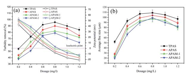
Fig. 9 Effect of the dosage on (a) turbidity removal and zeta potential, and (b) floc size.
