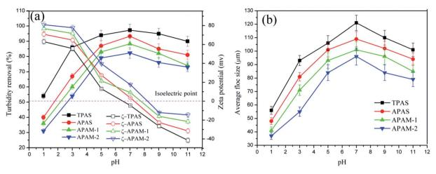
Fig. 10 Effect of the pH on (a) turbidity removal and zeta potential, and (b) floc size.
