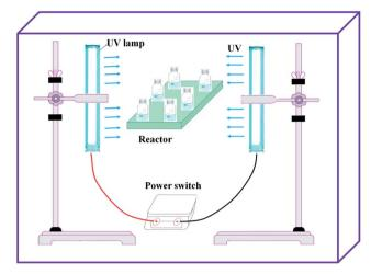
Fig. 2 The experimental setup of UV-initiated template copolymerization.
