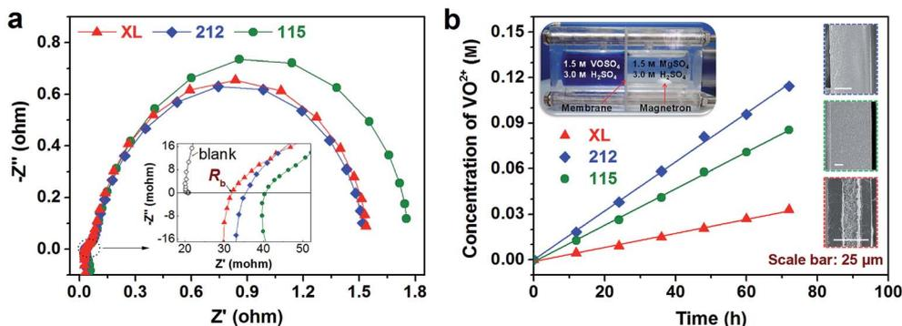
Fig. 3 Ion transport properties of various Nafion membranes: (a) Nyquist plots of VFBs assembled with various membranes, (b)  $\text{VO}^{2+}$  crossover plots (inset shows the cross-section SEM images of various membranes).
