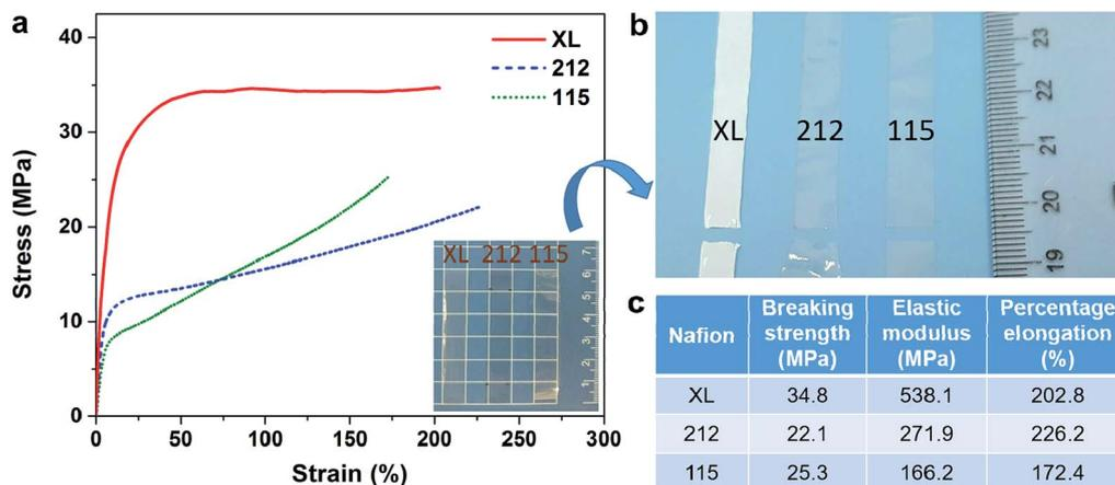
Fig. 2 Mechanical properties of various Nafion membranes: (a) strain–stress curves (inset shows the photograph of the samples before test), (b) photograph of the fracture, and (c) mechanical properties.
