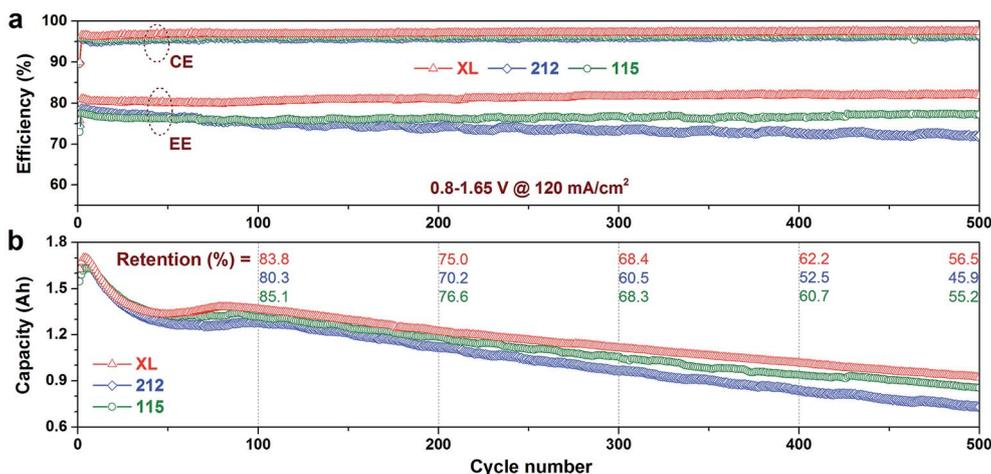
Fig. 6 Cycling performances of VFBs assembled with various Nafion membranes at current density of  $120 \text{ mA cm}^{-2}$ : (a) coulombic efficiency and energy efficiency, (b) discharge capacity and capacity retention.
