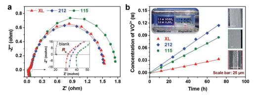
Fig. 3 Ion transport properties of various Nafion membranes: (a) Nyquist plots of VFBs assembled with various membranes, (b) VO<sup>2+</sup> crossover plots (inset shows the cross-section SEM images of various membranes).
