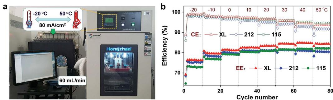
Fig. 8 All-climate performances of VFBS assembled with various Nafion membranes at current density of  $80 \text{ mA cm}^{-2}$ : (a) photograph of the test platform, (b) coulombic efficiency and energy efficiency as a function of temperature.
