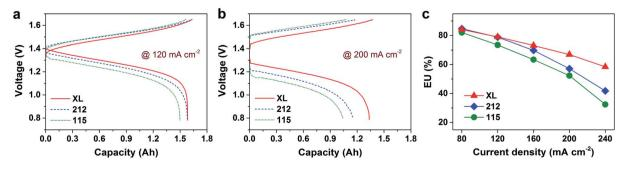
Fig. 5 Charge-discharge curves (a and b) and electrolyte utilization (c) of VFBs assembled with various Nafion membranes.
