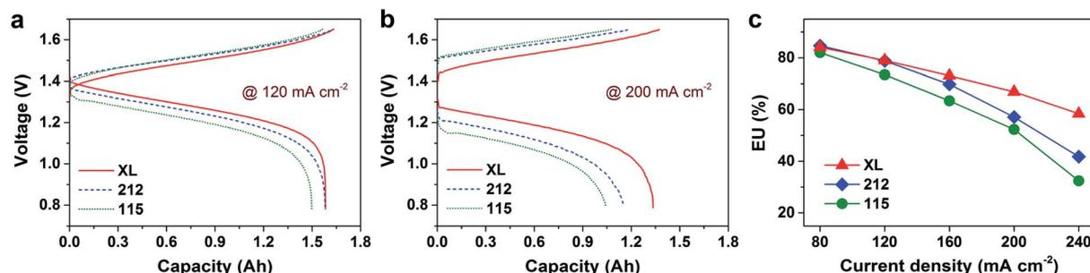
Fig. 5 Charge–discharge curves (a and b) and electrolyte utilization (c) of VFBs assembled with various Nafion membranes.
