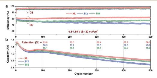
Fig. 6 Cycling performances of VFBs assembled with various Nafion membranes at current density of 120 mA cm<sup>-2</sup>: (a) coulombic efficiency and energy efficiency, (b) discharge capacity and capacity retention.
