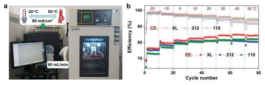
Fig. 8 All-climate performances of VFBs assembled with various Nafion membranes at current density of 80 mA cm $^{-2}$ : (a) photograph of the test platform, (b) coulombic efficiency and energy efficiency as a function of temperature.
