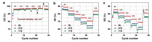
Fig. 4 Rate performances of VFBs assembled with various Nafion membranes: (a) coulombic efficiency, (b) voltage efficiency, (c) energy efficiency.
