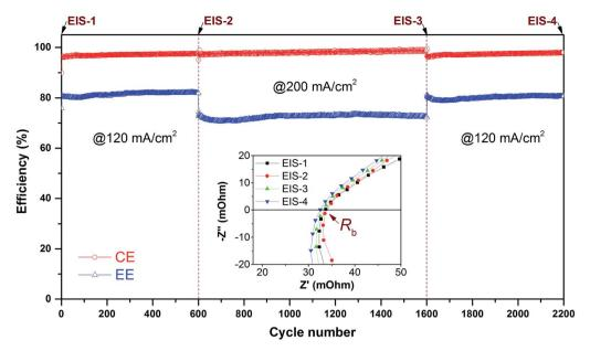
Fig. 7 Super long-term cycling stability of VFBs assembled with Nafion XL membrane. Inset shows the Nyquist plots of the initial VFB (EIS-1) and the VFB after 600 (EIS-2), 1600 (EIS-3), and 2200 (EIS-4) cycles.
