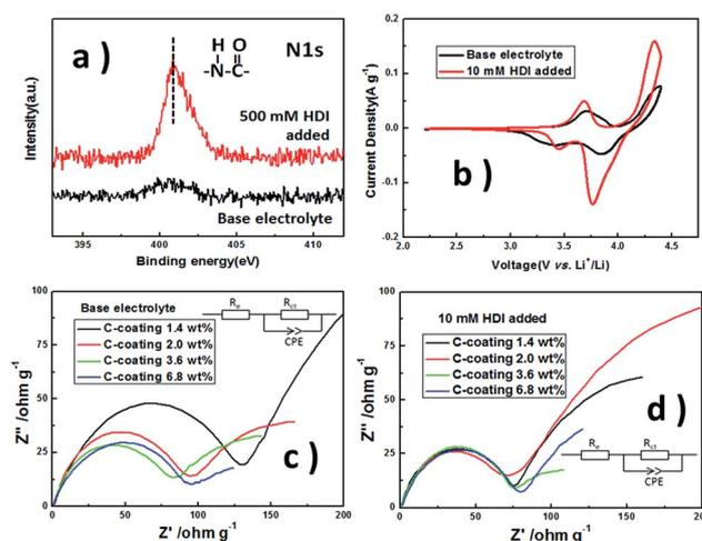
Fig. 2 XPS (a) and CV (b) spectra of  $\text{LiFe}_{0.2}\text{Mn}_{0.8}\text{PO}_4/\text{C}$  (2.0 wt%) cathodes in different electrolytes charged at 4.4 V (vs.  $\text{Li}^+/\text{Li}$ ) for 3 hours, scanned with  $0.1 \text{ mV s}^{-1}$ . EIS of  $\text{Li}/\text{LiFe}_{0.2}\text{Mn}_{0.8}\text{PO}_4/\text{C}$  cells with different C-coatings in base (c) and 10 mM HDI added (d) electrolytes charged at 4.4 V (vs.  $\text{Li}^+/\text{Li}$ ) for 3 hours. The inset images are the simulated models.
