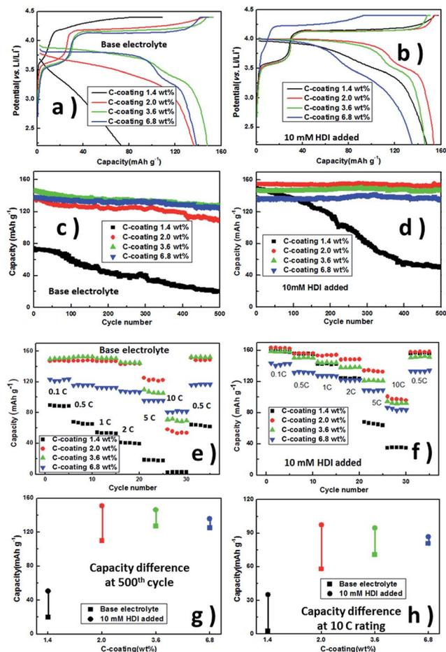
Fig. 3 The first charge–discharge curves (a and b), cycling (c and d) and rating (e and f) performances of Li/LiFe<sub>0.2</sub>Mn<sub>0.8</sub>PO<sub>4</sub>/C cells with different C-coatings in base and 10 mM HDI added electrolytes at RT, and the capacity difference (g and h) between cells with and without HDI added at the 500th cycle and 10C rating.
