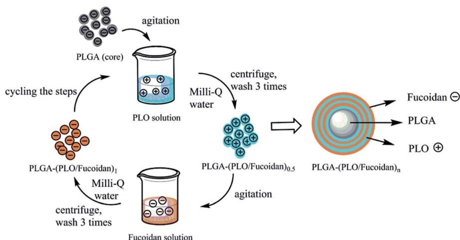
Fig. 3 Schematic illustration of preparation steps of PLGA-(PLO/fucoidan)<sub>n</sub> nanoparticles by ultrasonic emulsification of LbL self-assembly.
