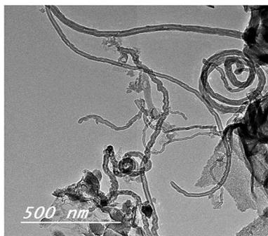
Fig. 8 TEM image of the prepared CNTs from hydrothermal carbonization of RS-H/Fe-Ni.
