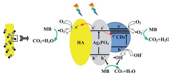
Fig. 10 Photocatalytic mechanisms for MB degradation by HA/N-CDs/Ag<sub>3</sub>PO<sub>4</sub>.
