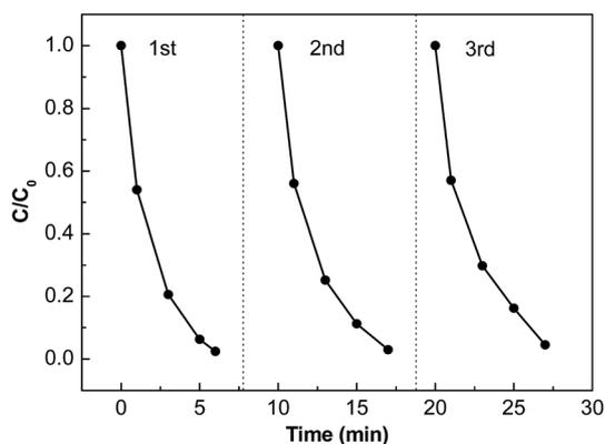
Fig. 8 Recycle experiments of MB degradation by HA/N-CDs/Ag<sub>3</sub>PO<sub>4</sub>-c.
