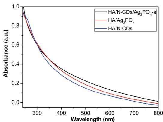
Fig. 5 UV/Vis absorption spectra of HA/N-CDs, HA/Ag<sub>3</sub>PO<sub>4</sub> and HA/N-CDs/Ag<sub>3</sub>PO<sub>4</sub>-a.
