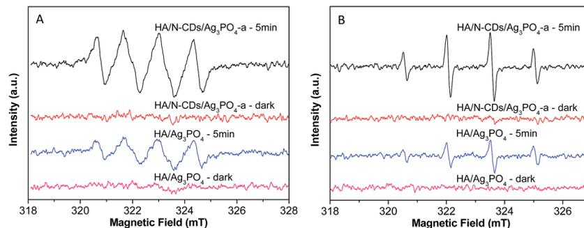
Fig. 9 ESR signals of HA/Ag<sub>3</sub>PO<sub>4</sub> and HA/N-CDs/Ag<sub>3</sub>PO<sub>4</sub>-a: (A)  $\cdot\text{O}_2^-$  and (B)  $\cdot\text{OH}$ .
