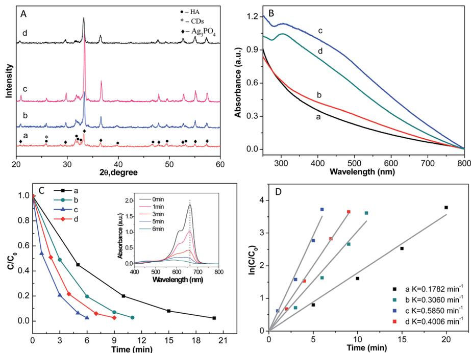
Fig. 7 (A) XRD patterns of HA/N-CDs/Ag<sub>3</sub>PO<sub>4</sub> with different silver loading amount, (B) UV/Vis absorption spectra, (C) photocatalytic activities, and (D) plots of  $\ln(C/C_0)$  versus irradiation time ( $t$ ).
