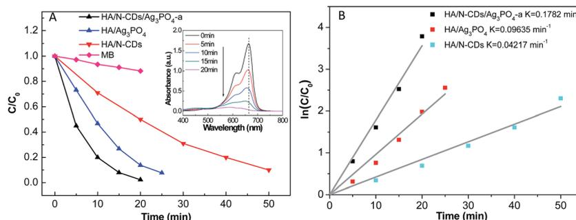
Fig. 6 (A) Photocatalytic activities of HA/N-CDs, HA/Ag<sub>3</sub>PO<sub>4</sub> and HA/N-CDs/Ag<sub>3</sub>PO<sub>4</sub>-a for MB degradation under visible-light irradiation, and (B) plots of  $\ln(C/C_0)$  versus irradiation time ( $t$ ).
