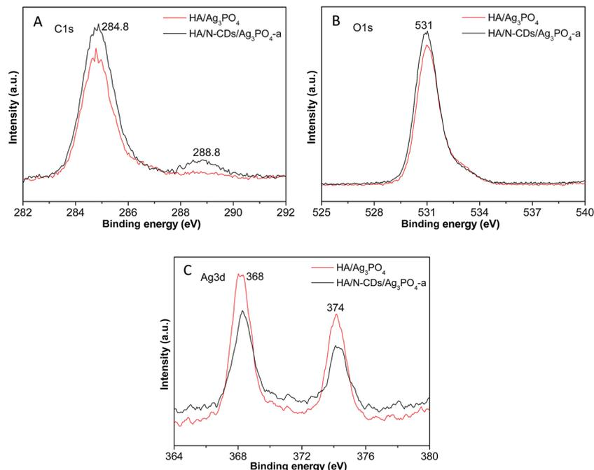
Fig. 4 XPS spectra of HA/Ag<sub>3</sub>PO<sub>4</sub> and HA/N-CDs/Ag<sub>3</sub>PO<sub>4</sub>-a: (A) C1s, (B) O1s and (C) Ag3d.
