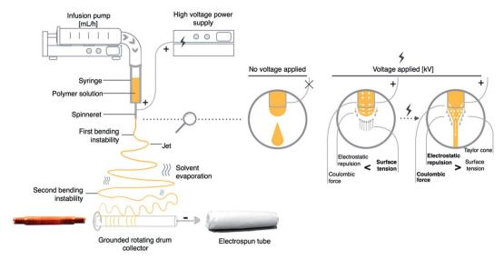
Fig. 1 Scheme of basic electrospinning setup for vascular graft preparation with a graphic representation of the effect of high voltage on electrospun polymer solution.
