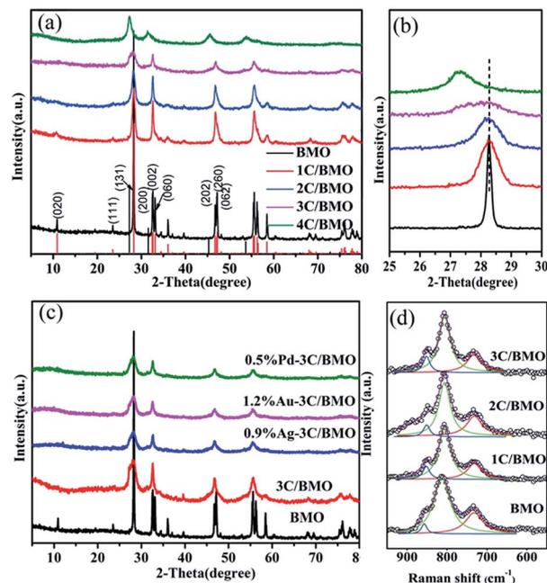
Fig. 1 XRD pattern (a and b), Raman spectra (d) of pristine Bi<sub>2</sub>MoO<sub>6</sub> and carbonate doped Bi<sub>2</sub>MoO<sub>6</sub> and XRD patterns of various noble metals loaded on 3C/BMO (c). Vertical bars in (a) indicate the standard data for Bi<sub>2</sub>MoO<sub>6</sub> (JCPDS card no. 77-1246, red line) and Bi<sub>2</sub>O<sub>3</sub> (JCPDS card no. 16-0654, black line).
