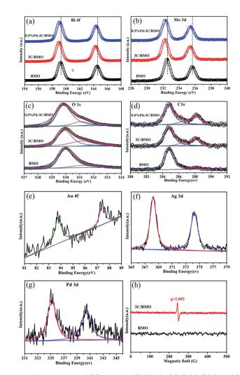
Fig. 2 High-resolution XPS spectra of Bi (a), Mo (b), O (c), C (d), Au (e), Ag (f), Pd (g) and ESR spectra (h) at room temperature.
