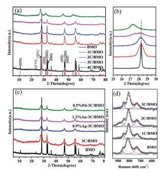
Fig. 1 XRD pattern (a and b), Raman spectra (d) of pristine Bi<sub>2</sub>MoO<sub>6</sub> and carbonate doped Bi<sub>2</sub>MoO6 and XRD patterns of various noble metals loaded on 3C/BMO (c). Vertical bars in (a) indicate the standard data for Bi<sub>2</sub>MoO<sub>6</sub> (JCPDS card no. 77-1246, red line) and Bi<sub>2</sub>O<sub>3</sub> (JCPDS card no. 16-0654, black line).
