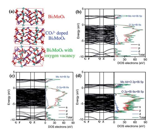
Fig. 6 Supercell structural models of  $Bi_2MoO_6$  used for calculation (a), band structures and the corresponding density of states of pure  $Bi_2MoO_6$ (b), CO<sub>3</sub><sup>2-</sup> doped Bi<sub>2</sub>MoO<sub>6</sub> (c) and Bi<sub>2</sub>MoO<sub>6</sub> with oxygen vacancy (d).
