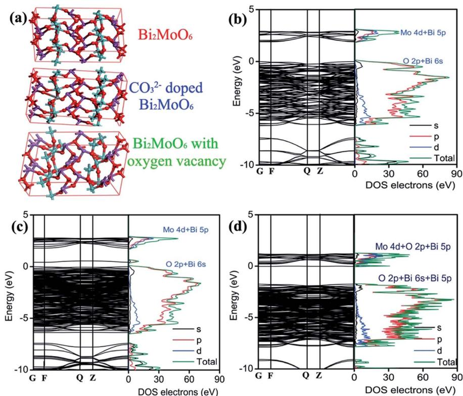
Fig. 6 Supercell structural models of  $\text{Bi}_2\text{MoO}_6$  used for calculation (a), band structures and the corresponding density of states of pure  $\text{Bi}_2\text{MoO}_6$  (b),  $\text{CO}_3^{2-}$  doped  $\text{Bi}_2\text{MoO}_6$  (c) and  $\text{Bi}_2\text{MoO}_6$  with oxygen vacancy (d).
