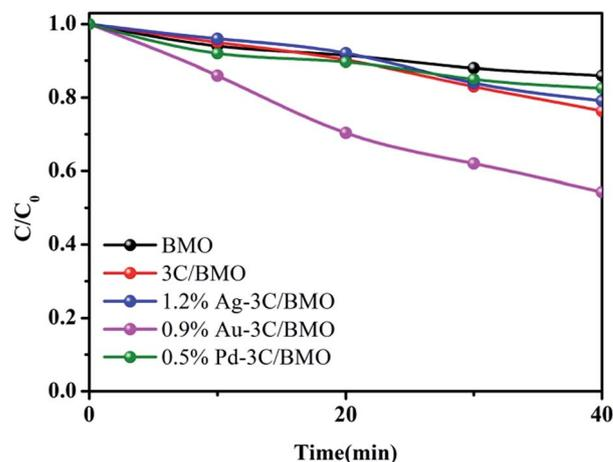
Fig. 9 The photocatalytic activities of pristine BMO, 3C/BMO as well as various noble metals loaded samples toward RhB degradation by using a bandpass filter (550 nm) with luminous power of 500 W.
