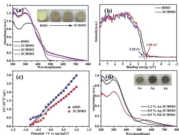
Fig. 5 UV-vis reflectance spectra of various samples (a). VB-XPS spectra of pristine BMO and 3C/BMO (b). Mott-Schottky plots of pristine BMO and 3C/BMO (c). UV-vis reflectance spectra of noble metals loaded on 3C/BMO (d). Inset figure reflects the colour of the as-prepared samples.
