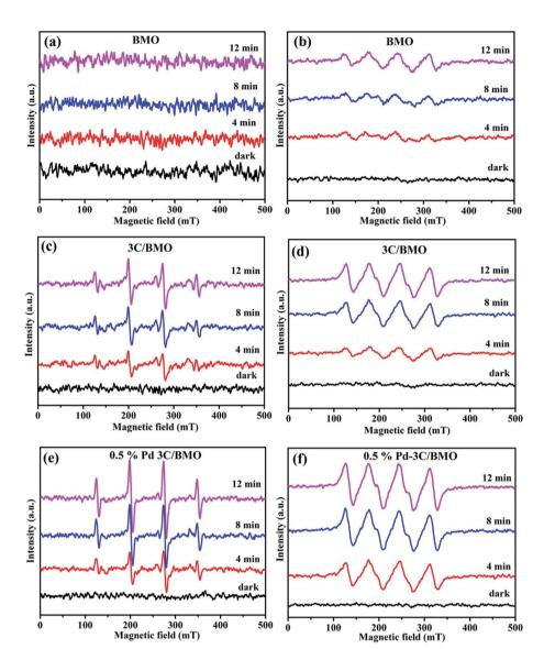
Fig. 12 ESR spectra of DMPO $^{\bullet}$ OH (a, c and e) and DMPO $^{\bullet}$ O $_2^{-}$  (b, d and f) adducts of pristine BMO, 3C/BMO and 0.5% Pd $^{-}$ 3C/BMO in darkness and under visible light irradiation with different irradiation times.
