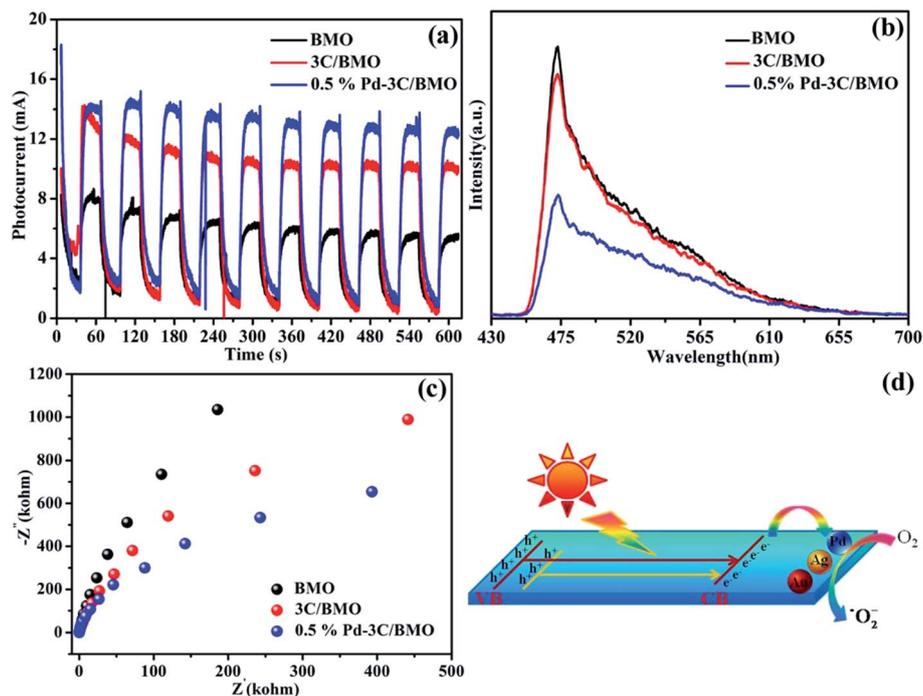
Fig. 13 Transient photocurrent responses (a), electrochemical impedance spectroscopy (b) and photoluminescence spectra (c) for pristine BMO, 3C/BMO and 0.5% Pd-3C/BMO. The mechanism illustration of 0.5% Pd-3C/BMO (d).
