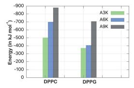
Fig. 7 At left, number of hydrogen bonds formed between water and peptides, with  $A_3K$  in green,  $A_6K$  in blue and  $A_9K$  in black. At right is the corresponding interaction energy of these peptides with the aqueous medium in kJ mol<sup>-1</sup>
