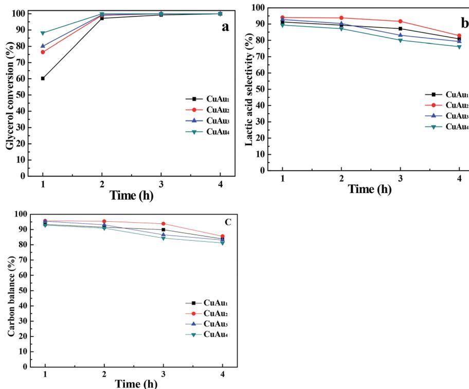
Fig. 4 Catalytic conversion of glycerol catalyzed by the bimetallic CuAu<sub>x</sub> nanoparticle catalysts. Reaction conditions: 100 mL of glycerol aqueous solution with the glycerol concentration of 2 mol L<sup>-1</sup>, NaOH/glycerol mole ratio of 1.1 : 1, 0.736 g of catalyst, and reaction temperature at 200 °C. (a) Glycerol conversion; (b) lactic acid selectivity; (c) carbon balance.
