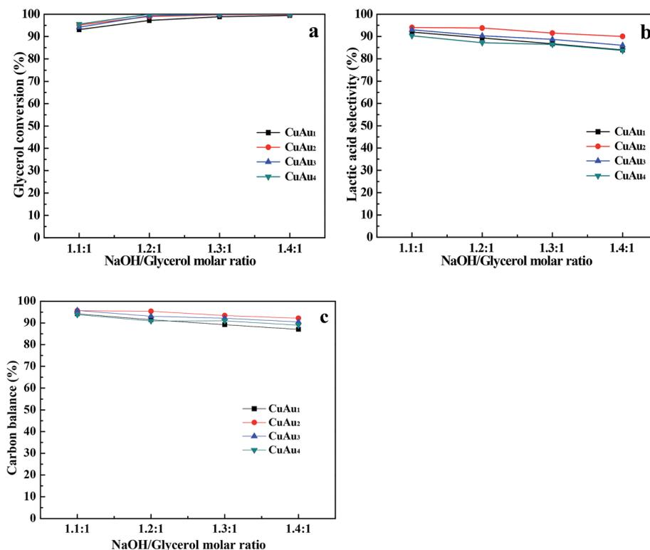
Fig. 6 Catalytic conversion of glycerol catalyzed by the bimetallic CuAu<sub>x</sub> nanoparticle catalysts. Reaction conditions: 100 mL of glycerol aqueous solution with the glycerol concentration of 2 mol L<sup>-1</sup>, 0.736 g of catalyst, reaction temperature at 200 °C, and reaction time of 2 h. (a) Glycerol conversion; (b) lactic acid selectivity; (c) carbon balance.
