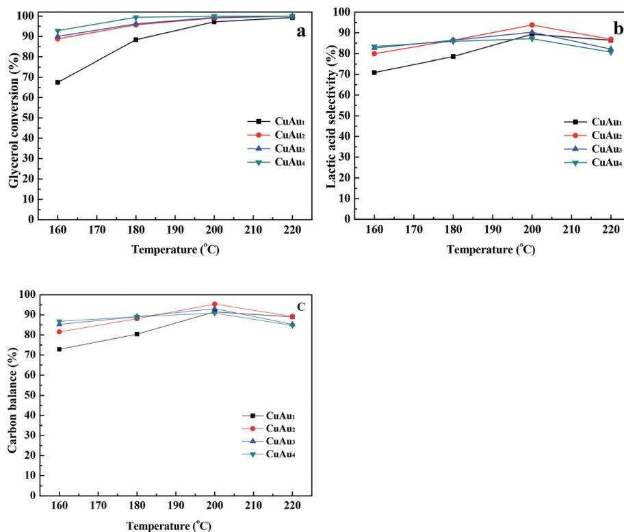
Fig. 5 Catalytic conversion of glycerol catalyzed by the bimetallic CuAu<sub>x</sub> nanoparticle catalysts. Reaction conditions: 100 mL of glycerol aqueous solution with the glycerol concentration of 2 mol L<sup>-1</sup>, NaOH/glycerol mole ratio of 1.1 : 1, 0.736 g of catalyst, and reaction time of 2 h. (a) Glycerol conversion; (b) lactic acid selectivity; (c) carbon balance.
