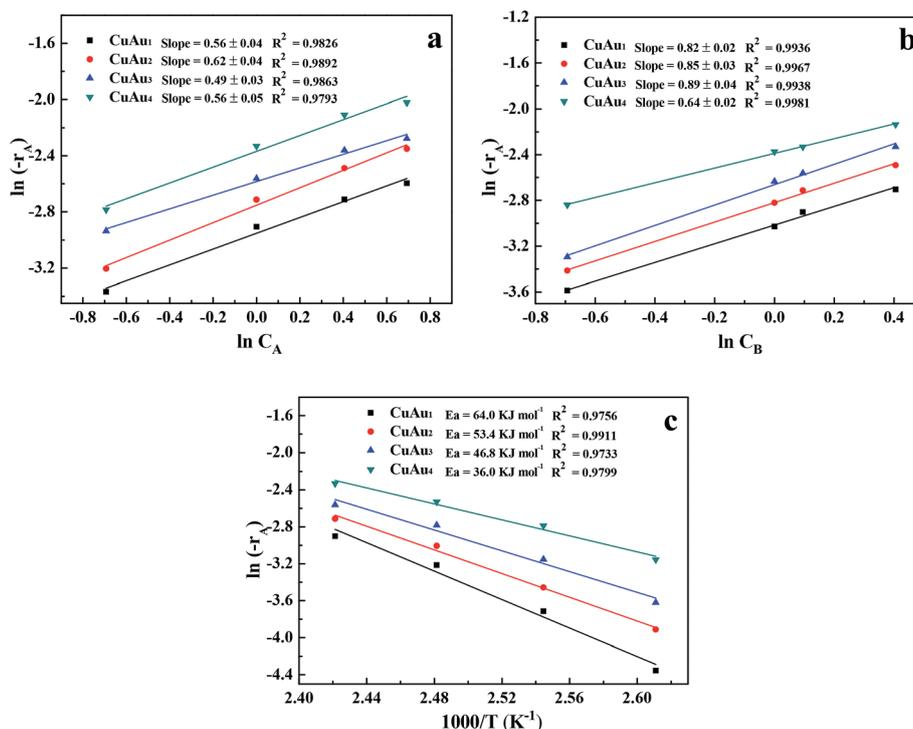
Fig. 8 Estimation of (a and b) the reaction orders and (c) the reaction activation energies for the power-function type reaction kinetics over the bimetallic  $\text{CuAu}_x$  nanoparticle catalysts.
