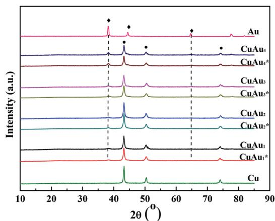
Fig. 1 XRD patterns of the monometallic Cu, monometallic Au, and fresh and spent bimetallic CuAu catalysts. ●, Cu<sup>0</sup>; ◆, Au<sup>0</sup>; \*, spent catalysts.
