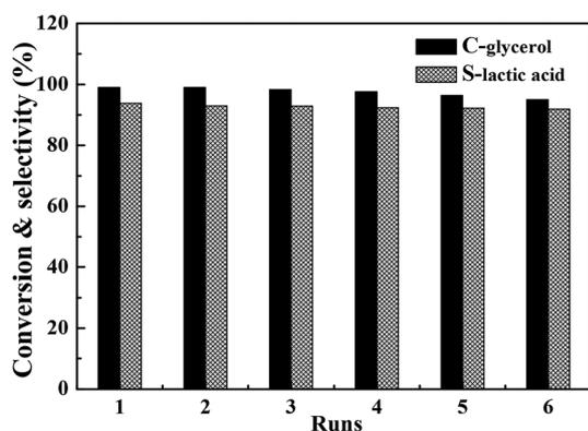
Fig. 7 Recycling performance of the bimetallic CuAu<sub>2</sub> nanoparticle catalyst. Reaction conditions for each run: 100 mL of glycerol aqueous solution with the glycerol concentration of 2 mol L<sup>-1</sup>; NaOH/glycerol mole ratio of 1.1 : 1; 0.736 g of catalyst; reaction temperature, 200 °C; reaction time, 2 h.
