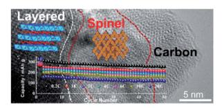
Fig. 11 A Li-rich LSC heterostructured cathode material, comprised of a Li-rich layered core, a spinel interlayer, and a carbon nanocoating Reproduced with permission.158
