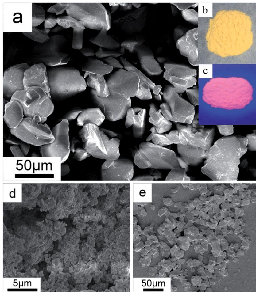
Fig. 2  $\text{K}_2\text{TiF}_6\text{:Mn}^{4+}$  red phosphor: (a) SEM image with typical photos illuminated under (b) natural and (c) 460 nm blue light. (d) and (e) are SEM images of  $\text{Na}_2\text{TiF}_6\text{:Mn}^{4+}$  and (c)  $\text{Cs}_2\text{TiF}_6\text{:Mn}^{4+}$  products.
