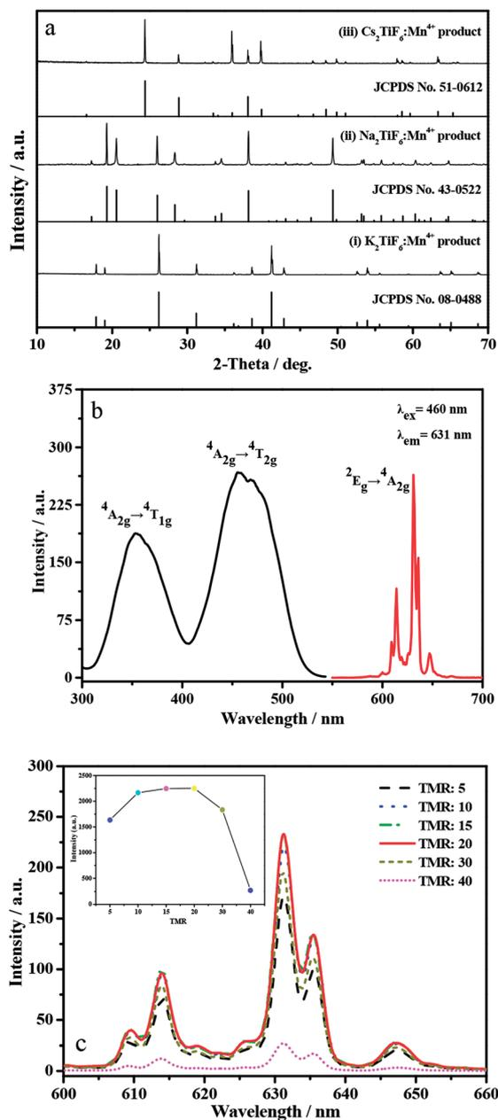
Fig. 1 (a) XRD patterns of (i)  $\text{K}_2\text{TiF}_6:\text{Mn}^{4+}$ , (ii)  $\text{Na}_2\text{TiF}_6:\text{Mn}^{4+}$  and (iii)  $\text{Cs}_2\text{TiF}_6:\text{Mn}^{4+}$ . (b) PLE and PL spectra of  $\text{K}_2\text{TiF}_6:\text{Mn}^{4+}$  product prepared with TMR of 20. (c) PL spectra of  $\text{K}_2\text{TiF}_6:\text{Mn}^{4+}$  product prepared with different TMRs. The inset figure of (c) shows the relationship between TMR and the relative integral emission intensity.
