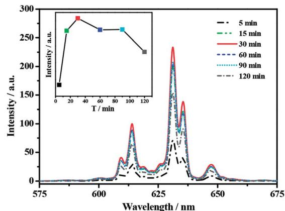
Fig. 3 PL spectra for  $\text{K}_2\text{TiF}_6\text{:Mn}^{4+}$  products prepared with different reaction time ( $\lambda_{\text{ex}} = 460 \text{ nm}$ ). The insert figure is the relationship between reaction time and relative integral emission intensity.
