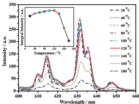
Fig. 4 Temperature-dependent emission spectra of  $\text{K}_2\text{TiF}_6:\text{Mn}^{4+}$  phosphor and relative intensity of emission spectrum by integrating the spectral area ( $\lambda_{\text{ex}} = 460$  nm).
