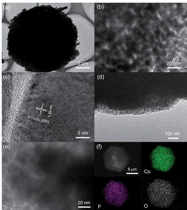
Fig. 3 (a and b) TEM images of layer-cake-like  $Co_3O_4$ , exhibiting porous structure consisting of nanoscale grains and voids. (c) High-resolution observation for  $Co_3O_4$ , showing a dominant (220) lattice plane. (d and e) TEM images of  $Co_3O_4/C$ , exhibiting a uniform carbon coating layer and maintaining a porous structure. (f) EDS element mapping of the layer-cake-like  $Co(OH)F$  precursor, confirming the existence of Co and F.
