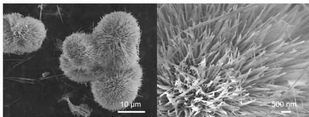
Fig. 2 Morphologies of pompon-like precursor obtained from the hydrothermal system with low  $F^-/Co^{2+}$  ratio, exhibiting average overall dimensions of about 10  $\mu m$  and radial nanowires (basic structural components) of 40–60 nm diameter.
