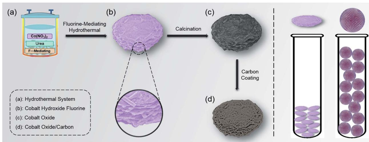
**Scheme 1** Left column: synthetic procedure: (a) fluorine-mediated homogeneous solution system. (b) Layer-cake-like Co(OH)F precursor with nano-micro hierarchical structure prepared via hydrothermal synthesis. (c) Co<sub>3</sub>O<sub>4</sub> obtained after calcination. (d) Co<sub>3</sub>O<sub>4</sub>/C obtained after carbon coating. Right column: comparison of simulated tap density between the layer-cake-like and pompon-like structures.
