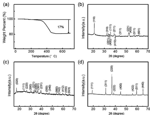
Fig. 4 (a) TG curve of Co(OH)F precursor. XRD patterns of (b) Co(OH)F precursor, (c) Co(CO<sub>3</sub>)<sub>0.5</sub>(OH)·0.11H<sub>2</sub>O precursor and (d) Co<sub>3</sub>O<sub>4</sub>/C final product.
